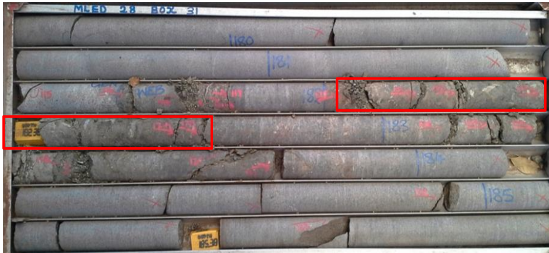
Figure 3-10. The alteration layer present in borehole core at Mine A (courtesy N. Fernandes).
