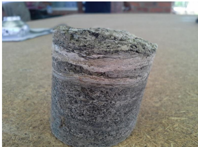
Figure 3-11. Core showing the striations that assist with the identification of the alteration layer during core logging (courtesy N. Fernandes).
