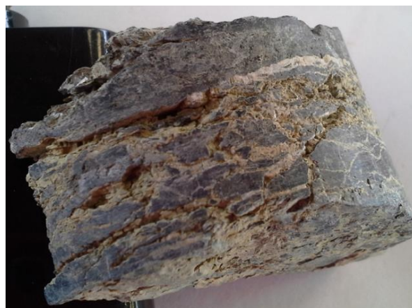
Figure 3-12. Alteration zone in borehole core with infilling and striations (courtesy N. Fernandes).
