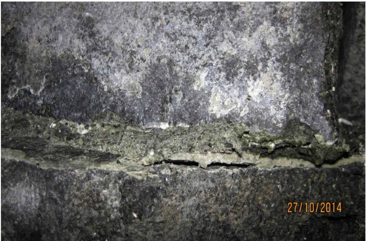
Figure 3-9. View of the alteration layer when weathered following exposure to moisture (courtesy N. Fernandes).
