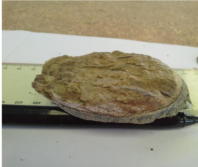
Figure 3-13. Mud-like texture and composition of the alteration zone from core drilling (courtesy N. Fernandes).
