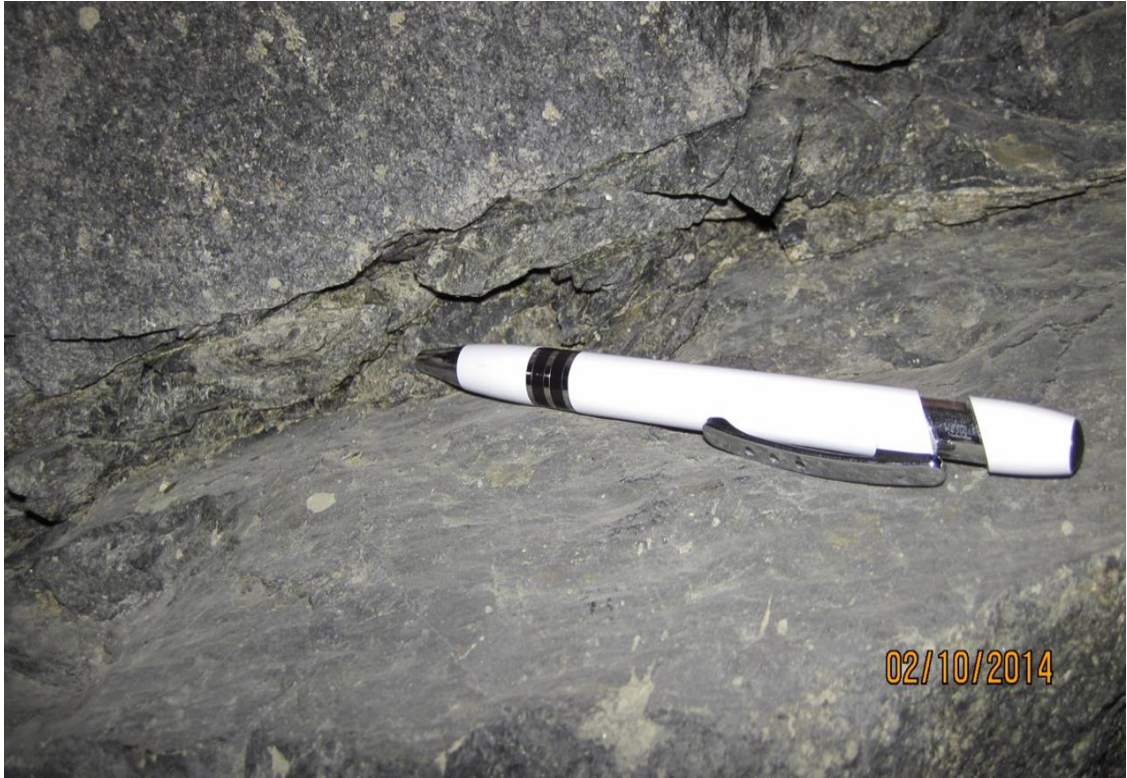
Figure 3-8. A close-up view of the alteration layer at Mine A (courtesy N. Fernandes).
