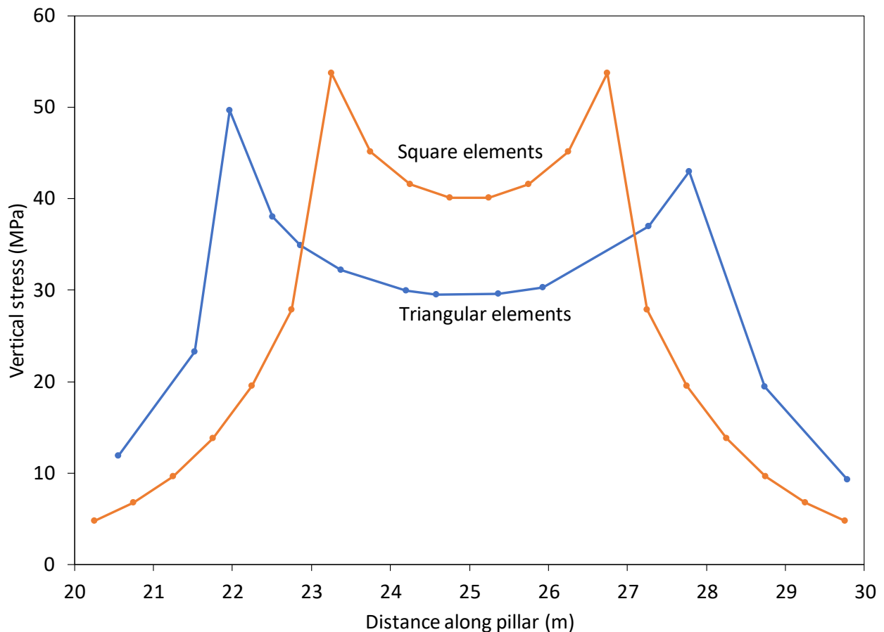
Figure 5-15. Vertical stress along section AA' for square and triangular element shapes.
