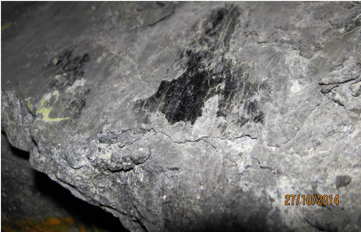
Figure 3-7. A close-up view of the alteration layer at Mine A illustrating the “slickenside” material (courtesy N. Fernandes).
