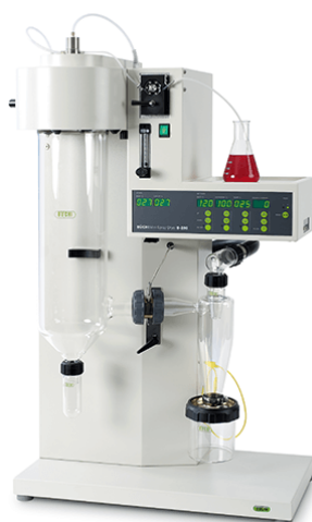
Figure 5.6: An image of a Büchi mini spray dryer used for spray-dried formulations [45].
