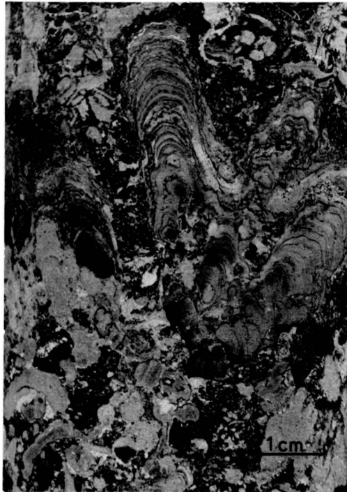
Figure 23: Stromatolitic, dolomitic limestone with black manganiferous areas and clastic infill between the stromatolites (AK520, RQ, Polo Ground Member, borehole core from Gopane mine).
