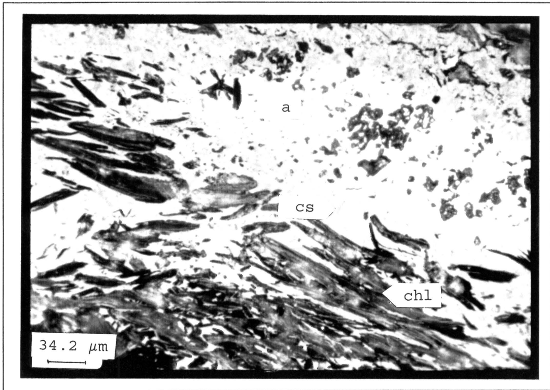
Fig. 6.11: Bi-Pb-Cu sulphosalt(a) rimmed by copper-sulphides(cs). The copper-sulphides replace the chlorite(chl); oil-immersion (GD2 at 15.85m).
