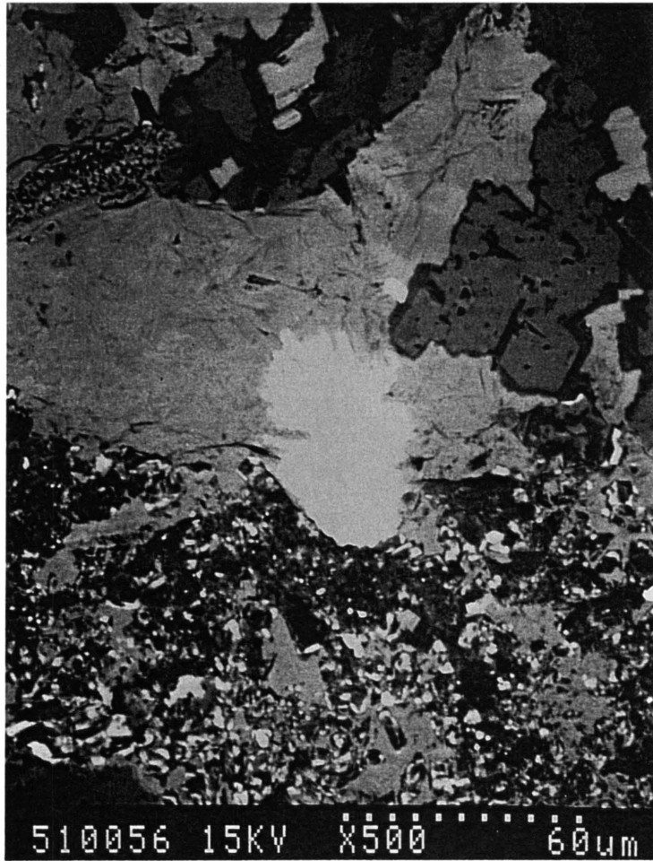
Figure 11.24 A rare-earth mineral (bright white) (back-scatter image 510056) is set in a large patch of chlorite (light grey), surrounded by zoned carbonate (darker to dark colours). The lower half of the back-scatter image displays smaller, rare-earth mineral grains. Back-scatter image (510055) is a magnification of the bright rare-earth mineral grain. The black sparry-like grains set in the rare-earth mineral grain are K-feldspar inclusions (sample KD111).
