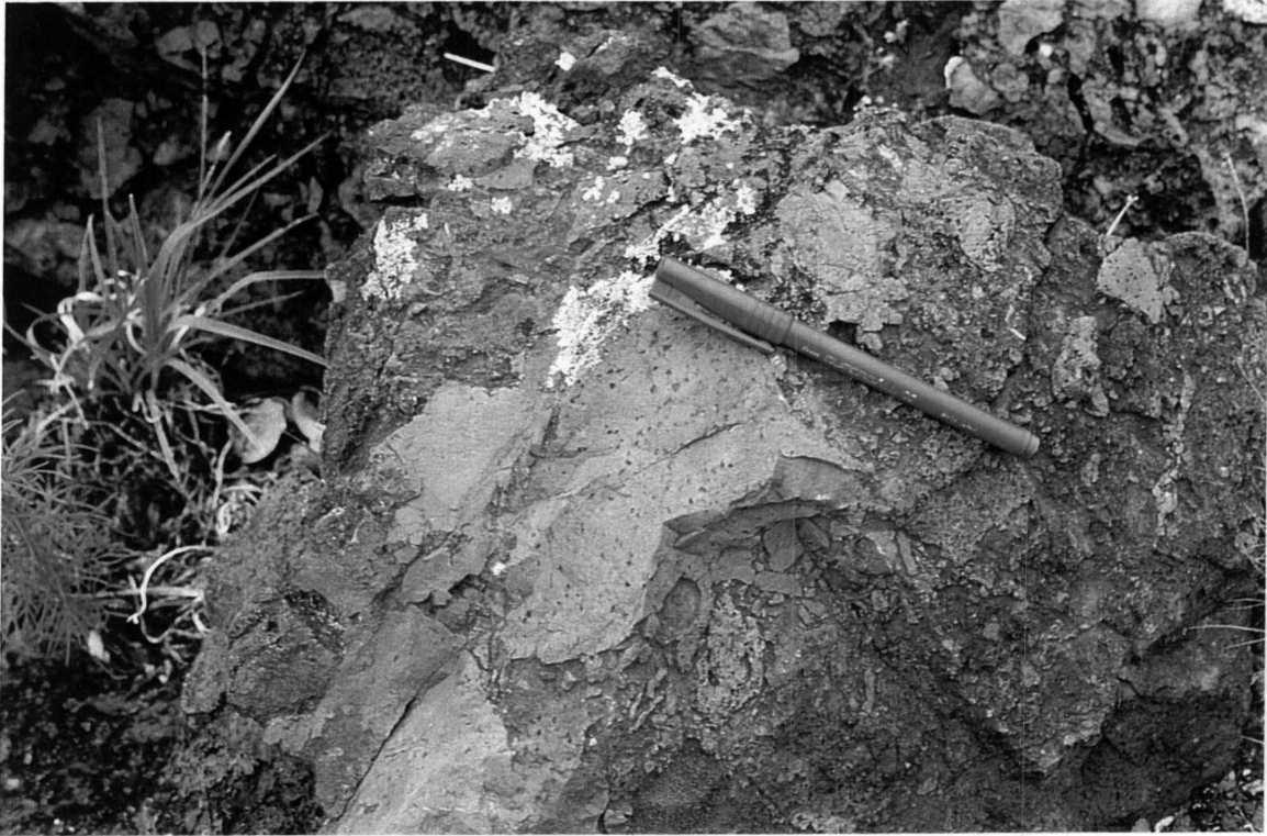
Figure 7.12 Large clasts in pyroclastic breccia (below the pen) consisting mainly of metasomatised material.
