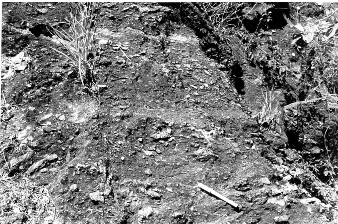
Figure 7.17 Poorly defined layering in a distal debris flow, displaying angular, matrix-supported clasts.
