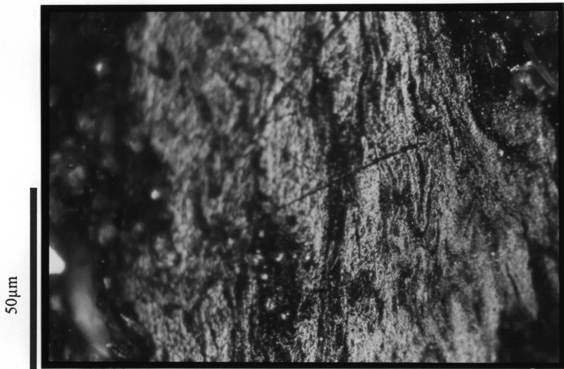
Figure 12. The surface of a filamentous carbonaceous particle in which the filaments are clearly visible.
