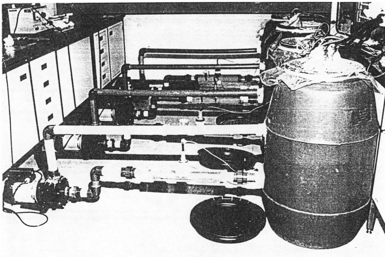
Figure 6.2 : Pilot rigs used for the evaluation of a linear polarisation corrosion monitoring device.
