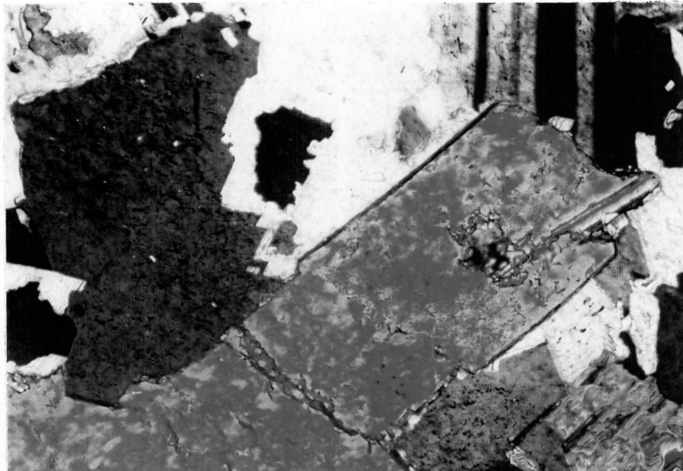
Fig 43 - Cassiterite-2, large, subhedral grain with predominantly magenta interference colour, replacing earlier-formed light buff-coloured ankerite. The grey to dark-grey minerals are feldspar and quartz of the arkosite. +N X200 Sample 250L7 A Mine - Jewel Box Section - 680' Level
