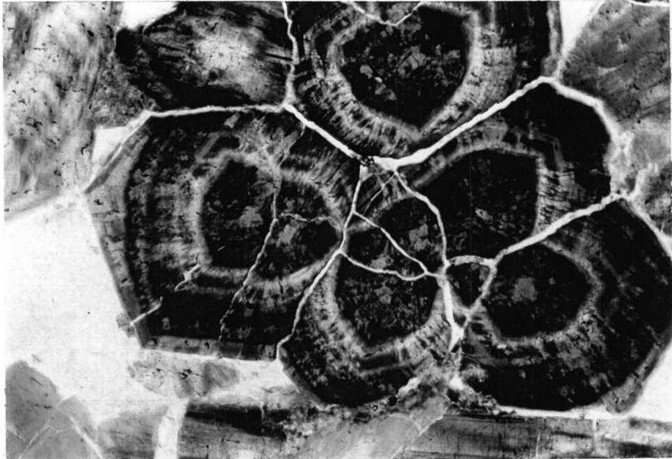
Fig. 26 - Zoning in tourmaline. Core dominated by the ditrigonal prism \{21\bar{3}0\} , modified by the trigonal prism \{10\bar{1}0\} ; overgrowth dominated by the hexagonal prism of the second order \{11\bar{2}0\} .
