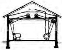
FIG. 2. Arrangement of belt drive in wash house.
