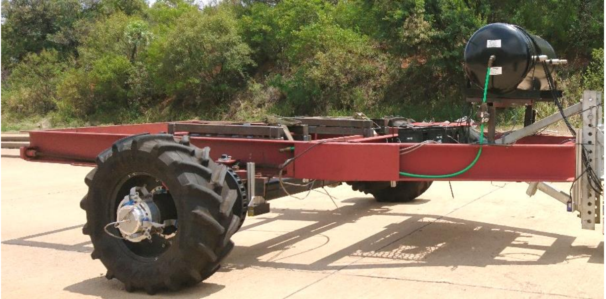
Figure 13: Damping Test Trailer fitted with TM700-280/70R16 tyres.
