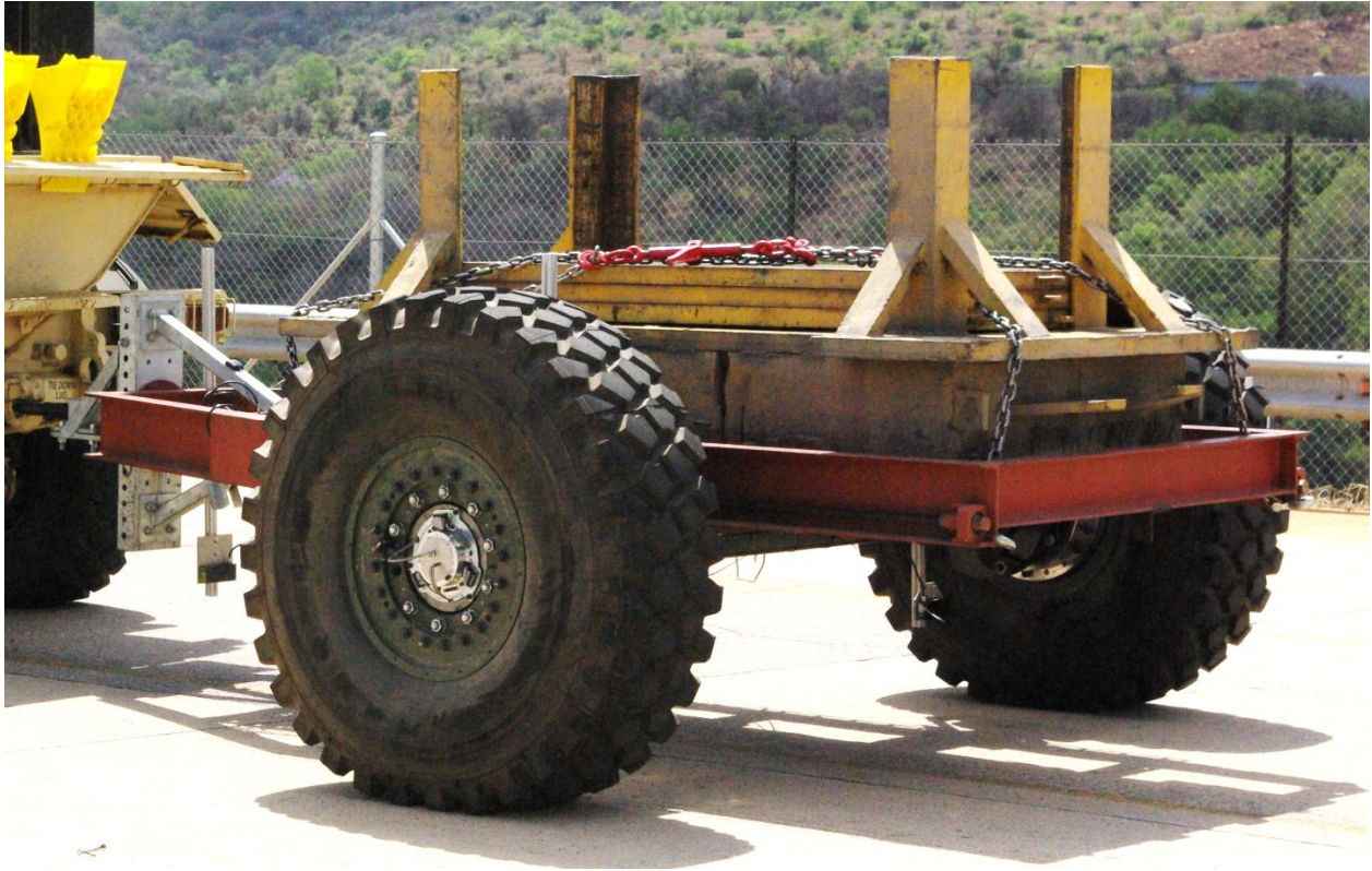
Figure 12: Damping Test Trailer from the Vehicle Dynamics Group at the University of Pretoria.
