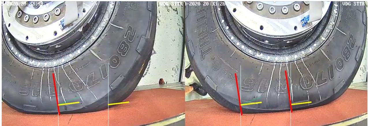
Figure 57: Sidewall tangential stiffness change at 150mm and 0mm longitudinal deflection, respectively from left to right at 0% tread and 80kPa inflation pressure.
