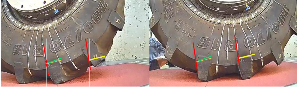
Figure 55: Tread deformation at 150mm and 0mm longitudinal deflection, respectively from left to right at 50% tread and 200kPa inflation pressure.
