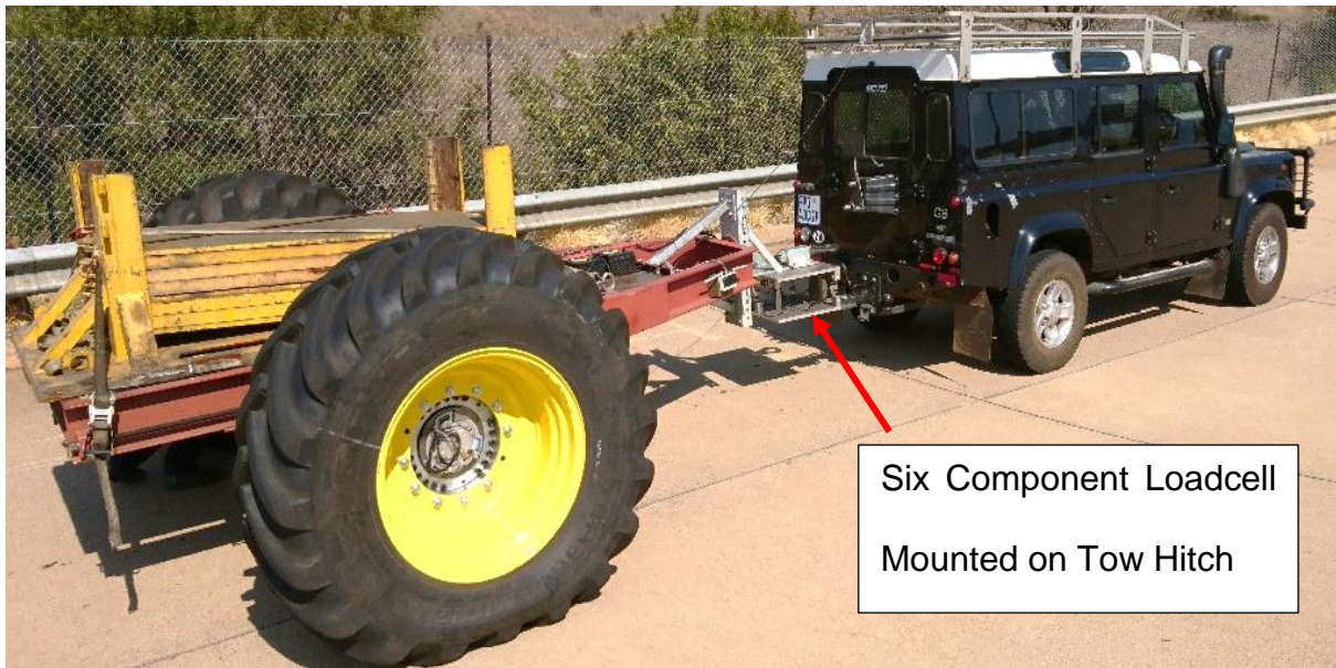
Figure 15: Motion resistance test setup for large tyres at high loads.
