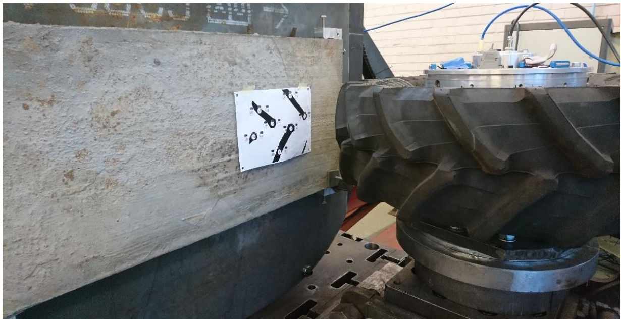
Figure 25: Microtexture profiling location template on STTR fitted with concrete test surface.
