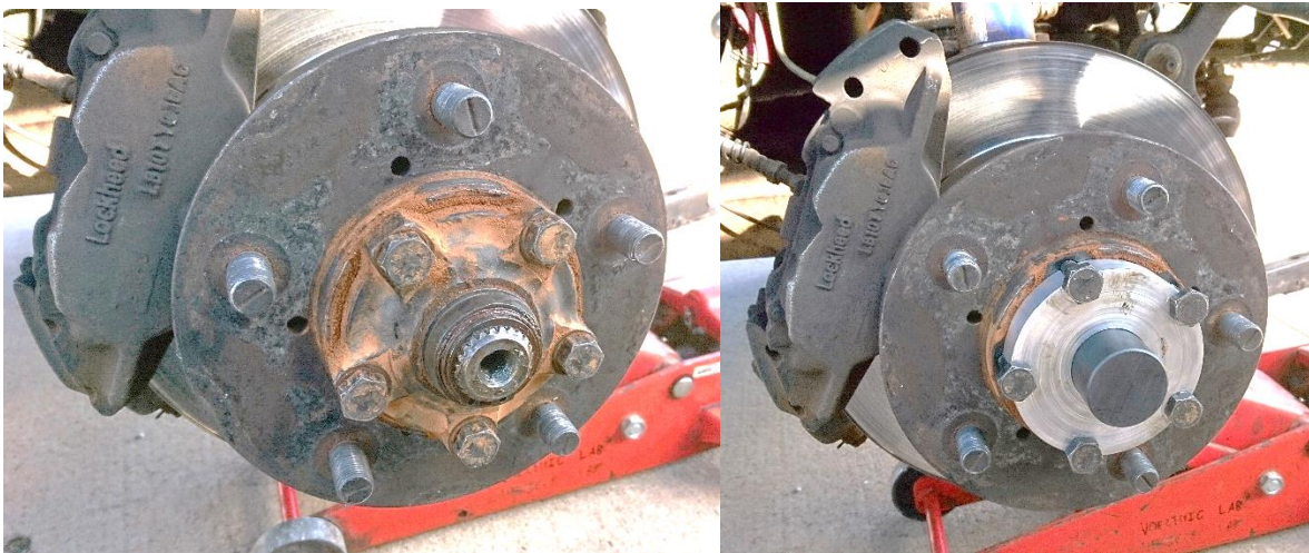
Figure 74: Standard splined spiders (left) and custom spineless spiders (right) on wheel hubs.
