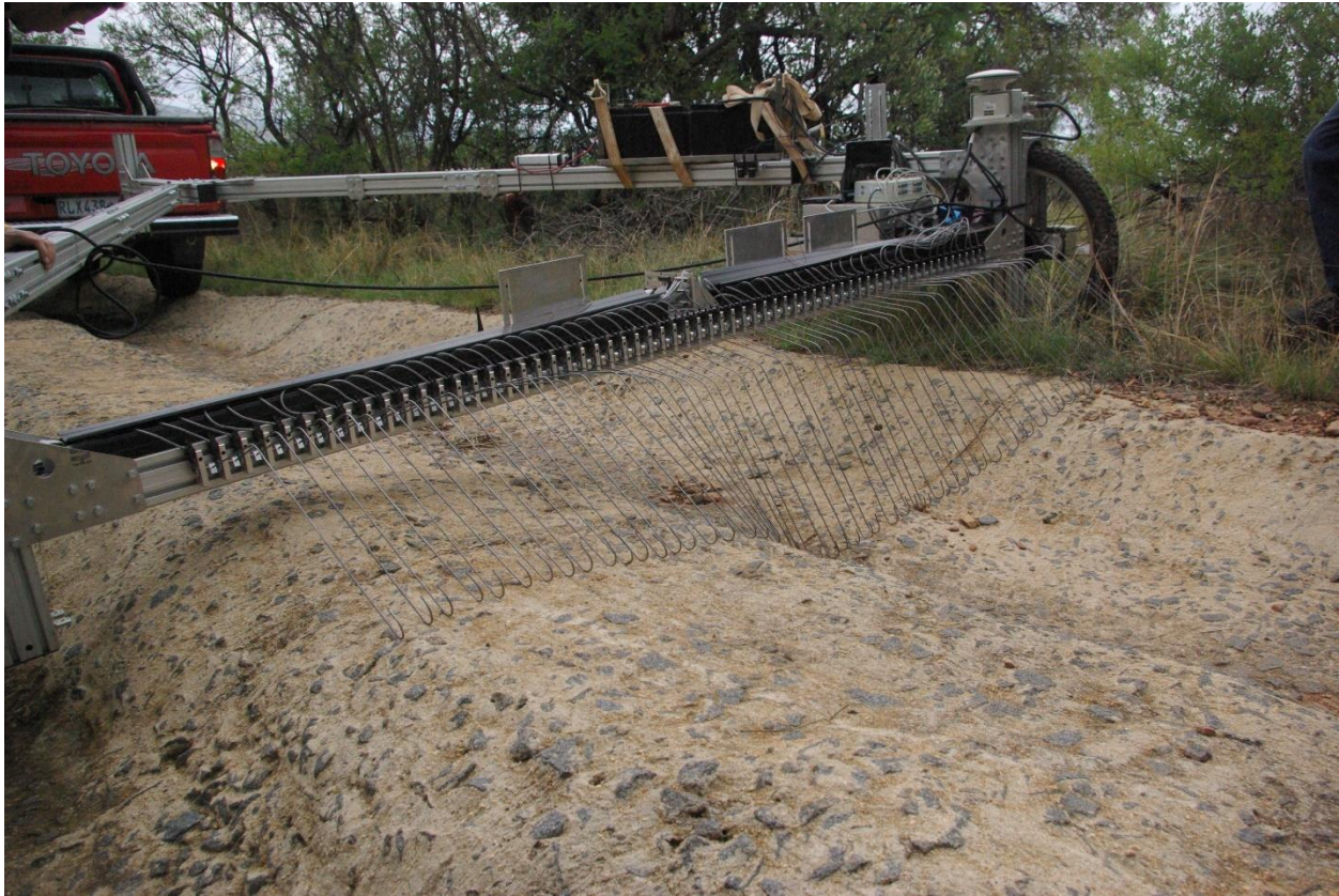
Figure 17: Can-Can machine profiling the rough track at Gerotek.
