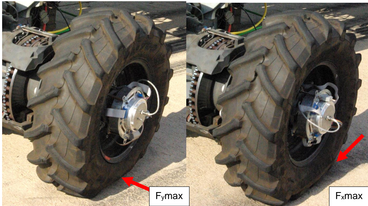
Figure 61: Friction envelope tests on Trelleborg TM700 280/70R16 at 11km/h, vertical load at 5.68kN before and during lockup at a constant lateral slip angle, respectively.
