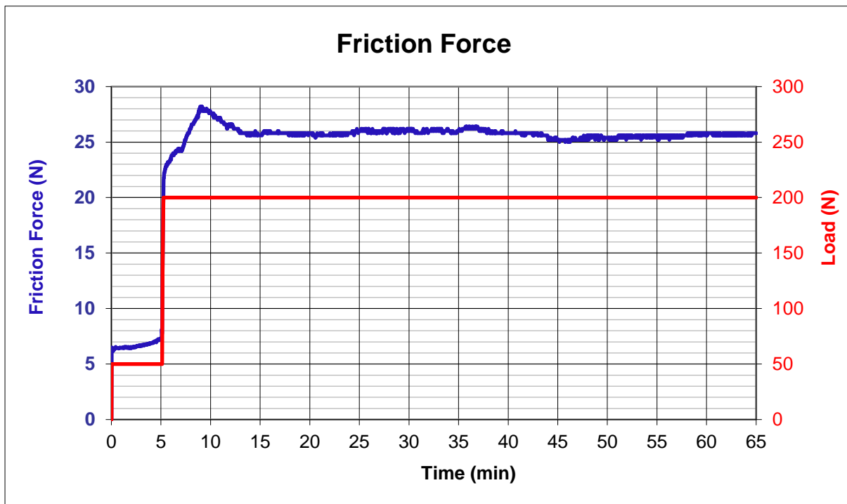
Figure 2.4: Example of friction force (blue curve) measured during a friction and wear test on the SRV test rig under lubricated conditions. The red graph is the applied load.
