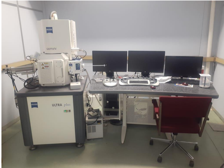
Figure 5. 2: High-resolution Zeiss Ultra, Plus 55 Scanning Electron Microscope.
