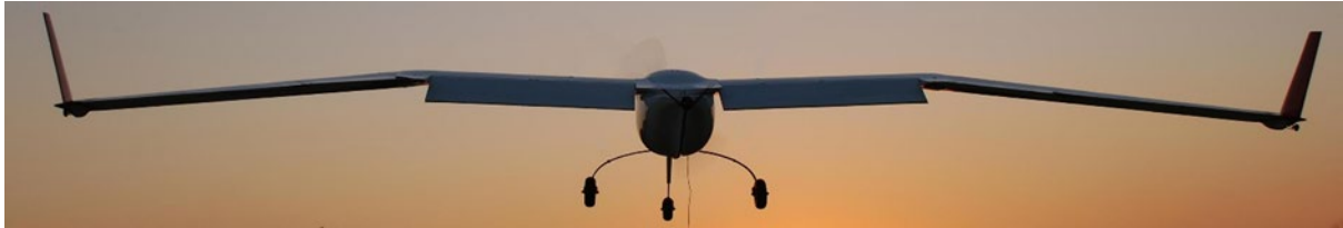
Figure E1 shows the motorised Exulans model with the flap set for landing. The \frac{1}{4} scale radio-controlled models shared a wing of 3 m span used on either a glider fuselage or on an electrically powered fuselage with tricycle gears, as seen here.
