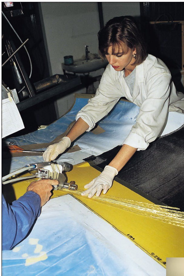
Figure F3 shows a hand lay-up in progress of the inner wing upper surface in a negative mould using a special resin dispenser. The carbon fibre in the D-box portion and the Kevlar in the rear wing skin can be seen after the outer layer of the sandwich was cured in a vacuum bag.
