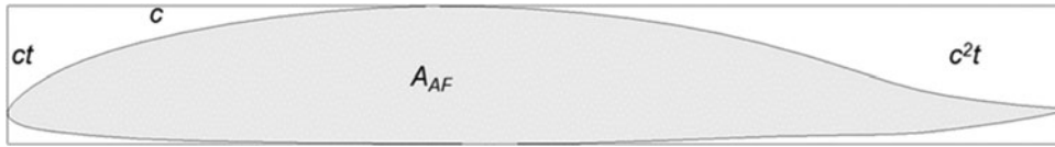
Figure 6. An aerofoil comparable to the DU97 of thickness t = 12.7\% has an area fraction f_{AF} = 68.4\% .
