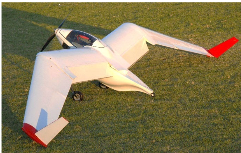
Figure E6 Note the fuselage aft body ready to be fitted with a fuselage trailing edge.
