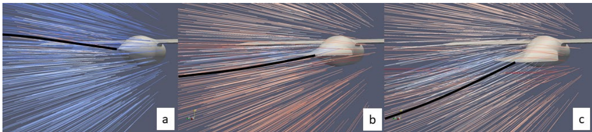
Figure 6.3 This set of pictures shows streamlines derived from the measured flow vectors using the visualisation tool, Paraview. Frame a) shows the body without a trailing edge and some upwash is visible in the wake. Frame b) and c) show progressive downward deflection of the trailing edge with increase of downwash in its wake.
