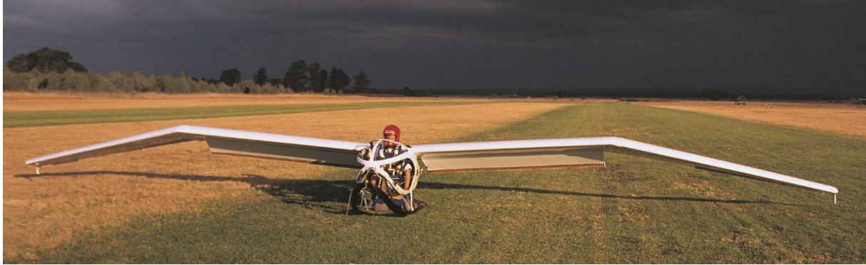
Figure F1 Exulans I resting on its landing skid on a glider runway while testing controls in a strong steady wind.
