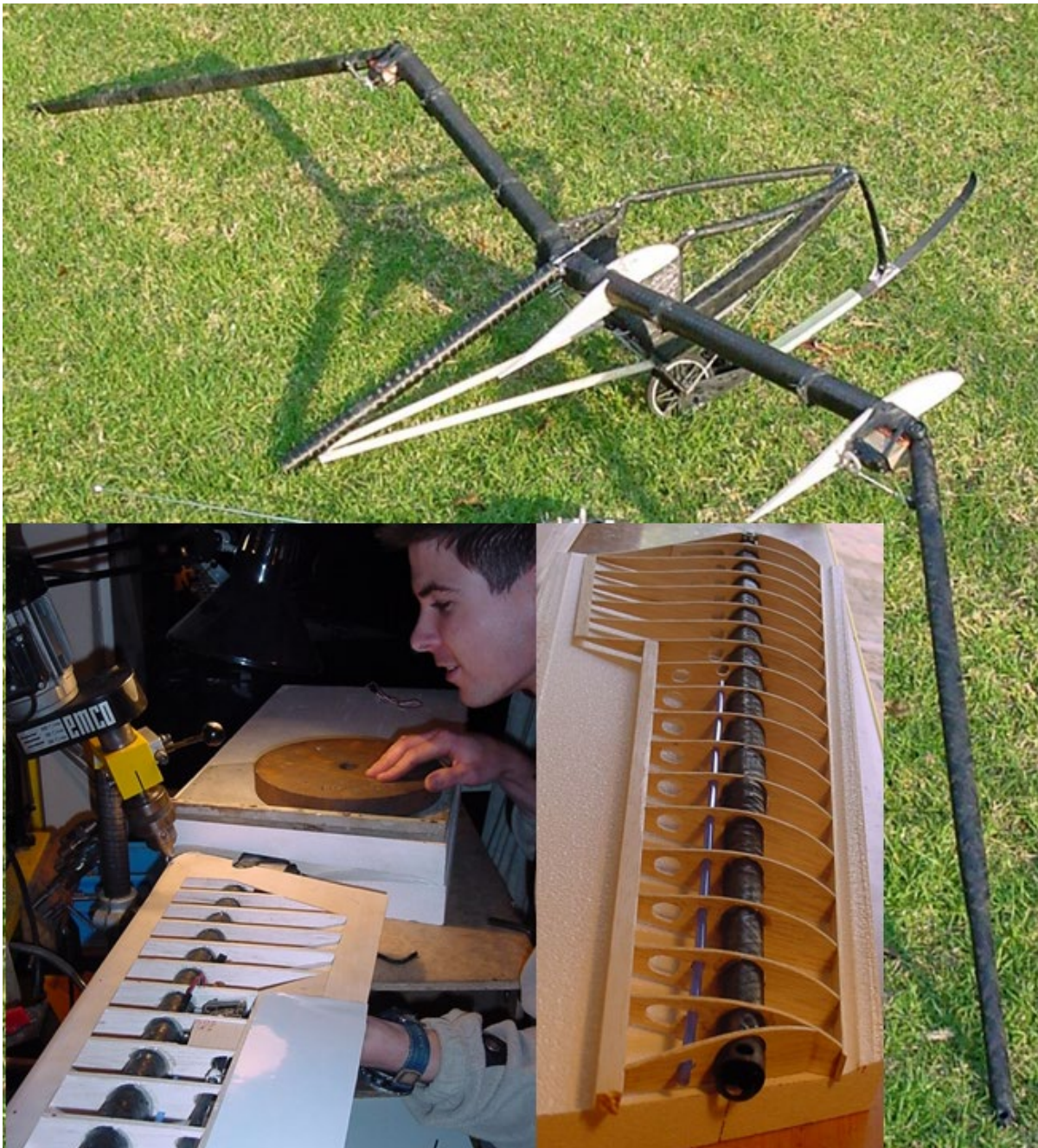
Figure E2 shows the primary skeletal wing and fuselage structure of the glider model and it shows how the tubular main spar was integrated into the wing. Here it can be seen how the primary tubular structure of the outer wing is integrated with balsa ribs to give the aerodynamic shape.
