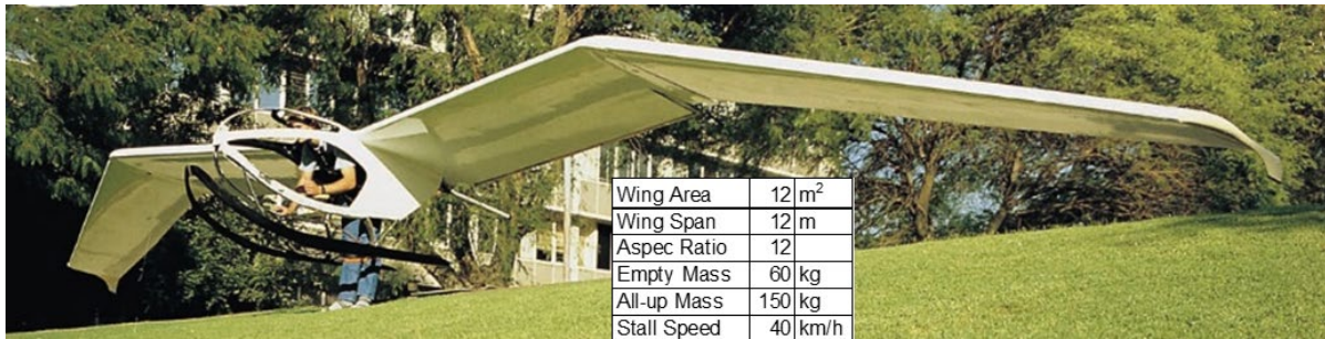
Figure F2 Exulans I as it would be carried by the pilot in the foot launch position.
