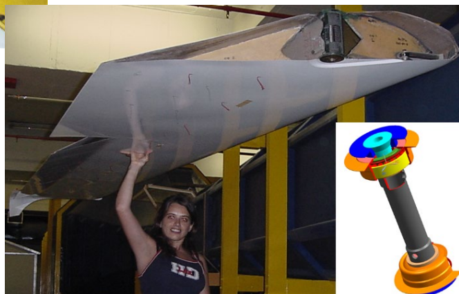
Figure F4 shows the outer wing of only 7 kg which included the wing sweep hinge (insert) of 0.8 kg.
