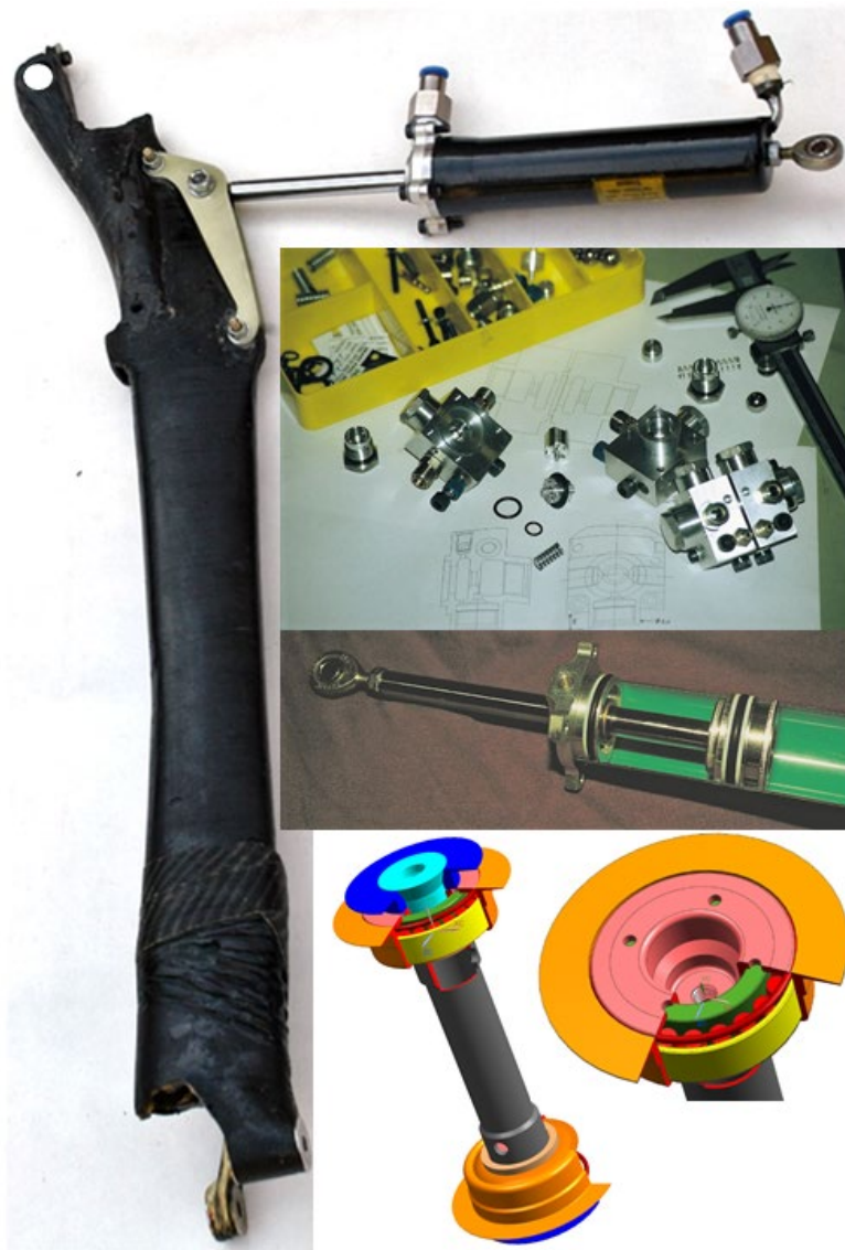
Figure F7 shows one of the pair of sweep levers with the input hydraulic cylinder which would be mounted in the cockpit. The pilot valves modules and a cut-away section of the carbon fibre hydraulic cylinder are also shown. The cutaway of the wing sweep hinge shows the roller bearing in the outer wing and shows the parts which join the inner wing.
