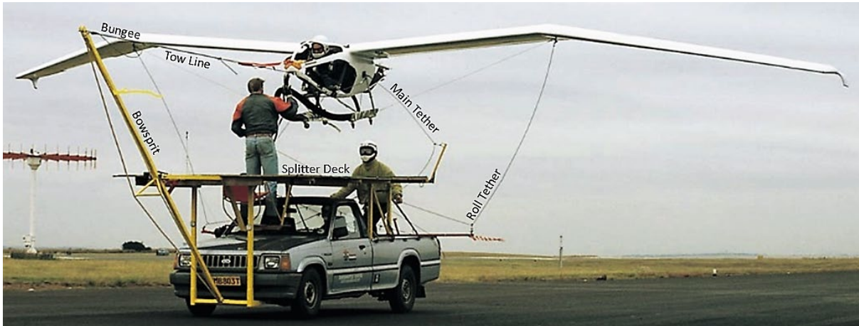
Figure 11 With the airspeed about 60 km/h the Exulans I is here flying about 4 m above the taxiway of the Swartkops air force Base, Pretoria, while the front operator is about to disturb the flight with a strong pitch input to simulate a gust.
