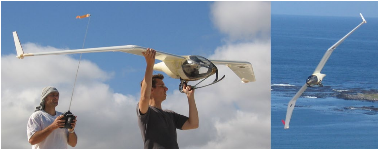
Figure E3 Here the glider is about to be hand-launched into a 10 m/s sea-breeze on a 100 m dune in the Cape in South Africa. These offered very turbulent flying conditions when close to terrain but the pilot had very responsive control to deal with such disturbances. Test manoeuvres would be flown away from the dune and when done the glider would be returned into the ridge-lift to recover lost height. Battery life or daylight rather than the wind would dictate the length of a flight once good wind conditions prevailed.
