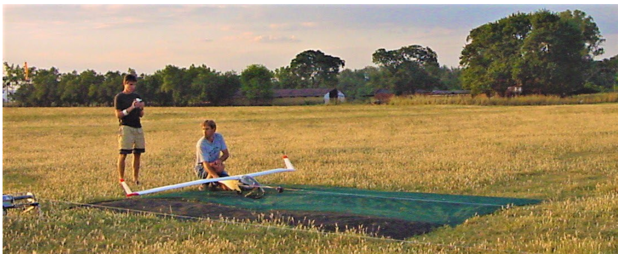
Figure E4 The model glider is hooked to a F3B winch by a Y link to a pair of CG hooks. After a short run on the ground cover the model would pitch up into an almost vertical climb.
