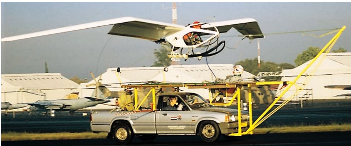
Figure 12 Exulans I flying over the splitter deck with flaps down in the landing setting. The front operator is sitting with a slack nose rope in his hand. Also the tether operator, hardly visible in the back minimises his flow obstruction by retreating below the deck while he ensures that the tethers are slack.
