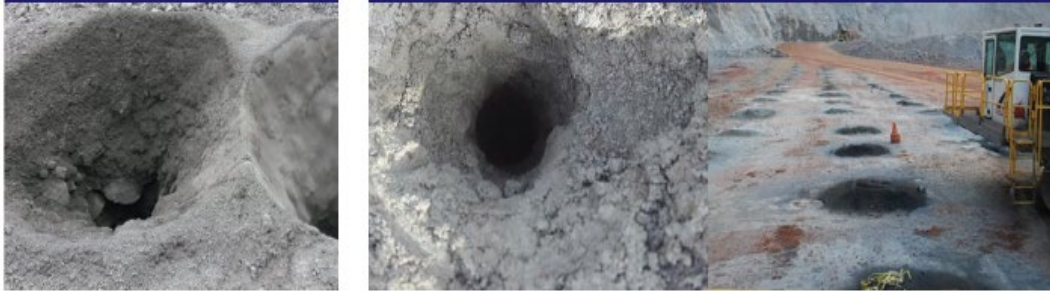
Figure 105 Drill collaring errors
