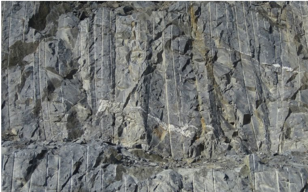
Figure 106 An example to drill deviation (source: Mining Magazine, 13 Feb 2015)
