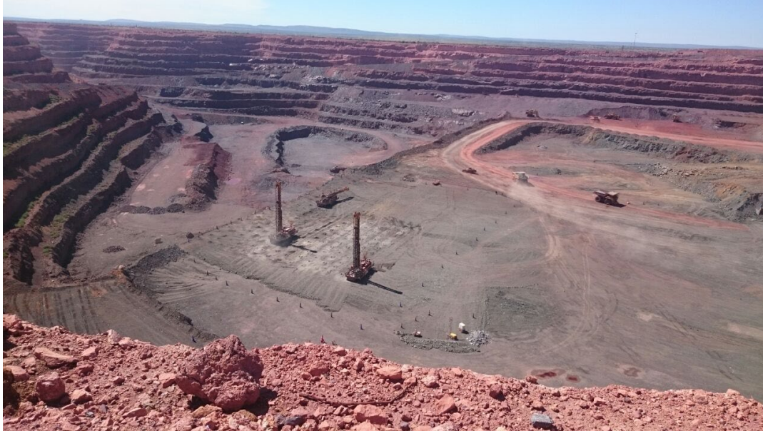
Figure 107 A view of a drilling block with three drill rigs allocated to it.
