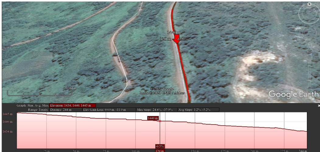
Figure 3-10: Google earth generated elevation profile of the Lunzua diversion canal section
