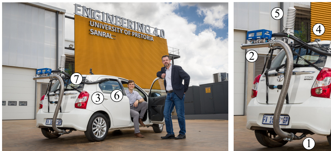
Figure 4.3: The SEMTECH ® DS+ PEMS unit fitted to a light vehicle from UP – a passenger car of the same vehicle class as the Ford Figo (UP, 2020).
