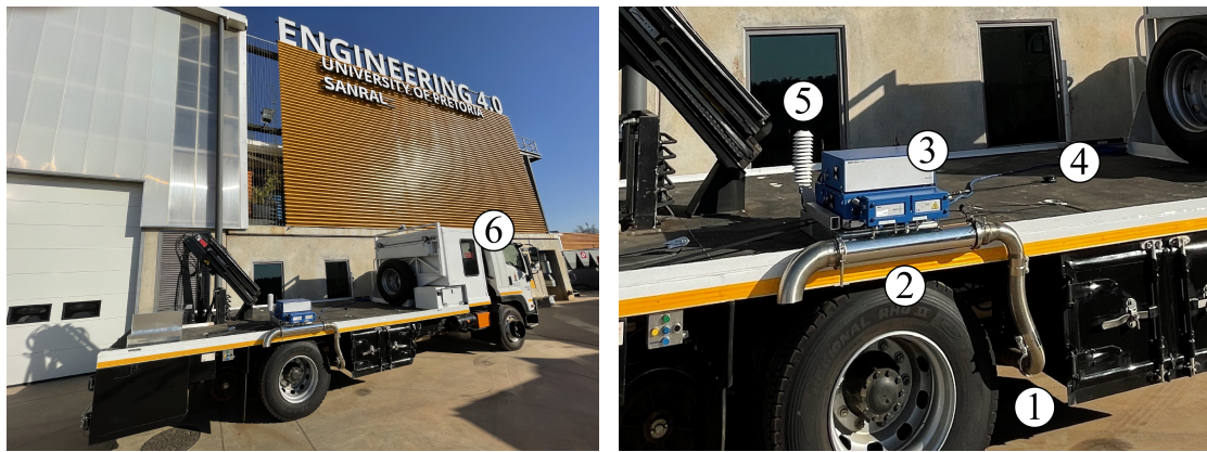
Figure 4.2: UP's Road Rail vehicle (RRV) fitted with the SEMTECH ® DS+ PEMS unit.
