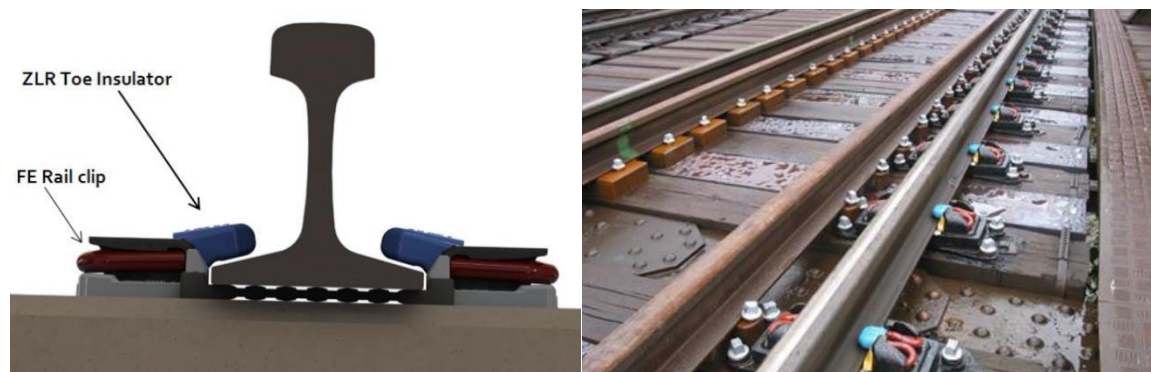
Figure 2.11: Example of ZLR's installed on rail bridge
