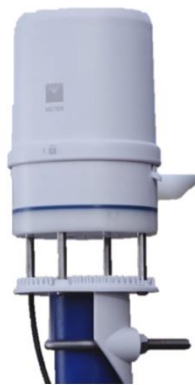
Figure 3.18: ATMOS 41 all-in-one weather station
