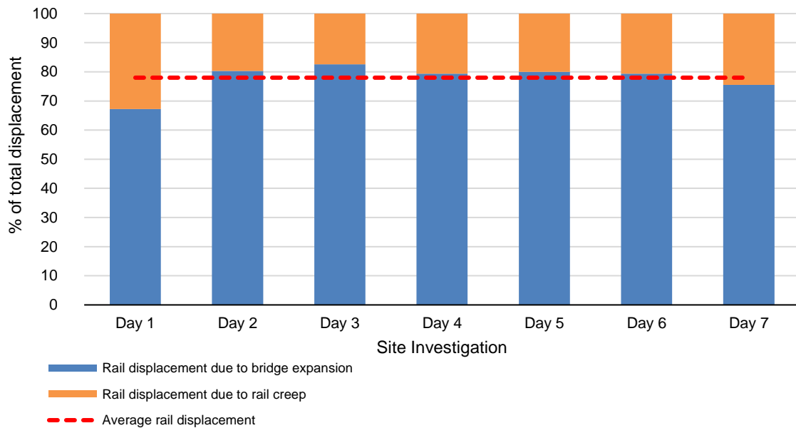
Figure 4.16: Rail displacement due to bridge expansion and rail creep (March 2019)
