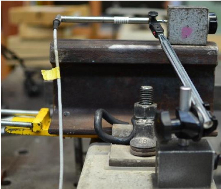
Figure 3.12: Example of longitudinal restraint test arrangement
