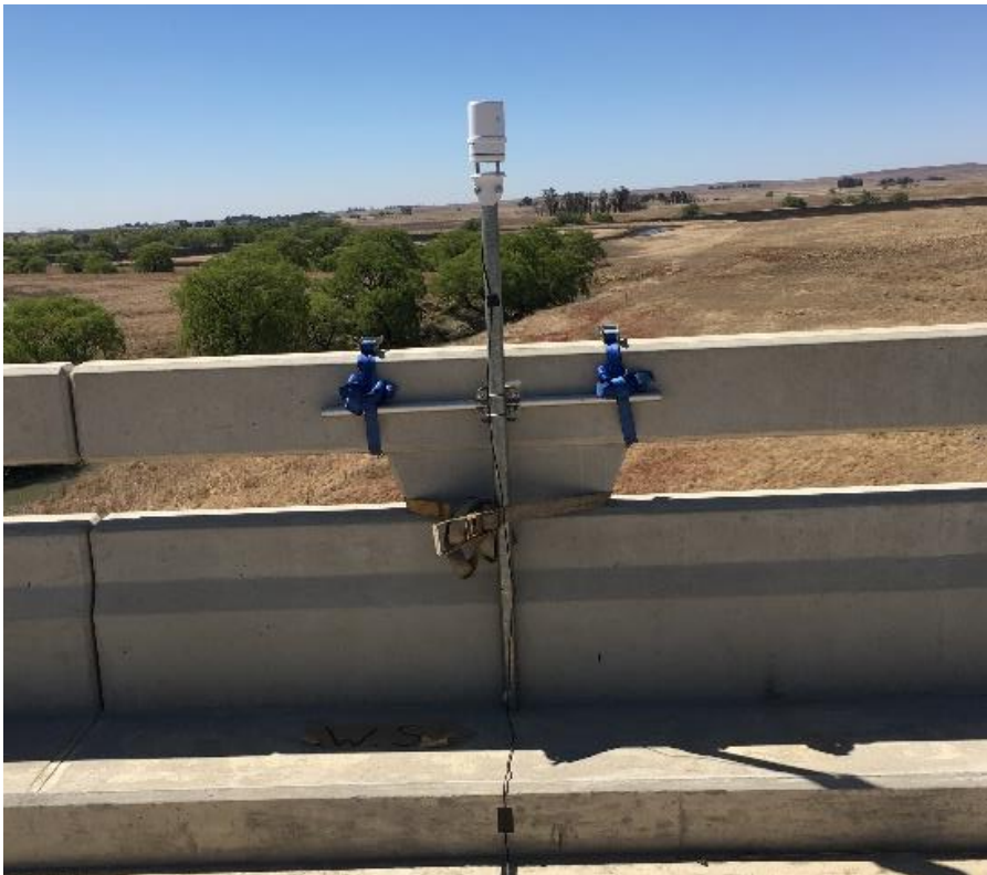
Figure 3.26: Site A - ATMOS 41 Weather Station (March 2018, September 2018)
