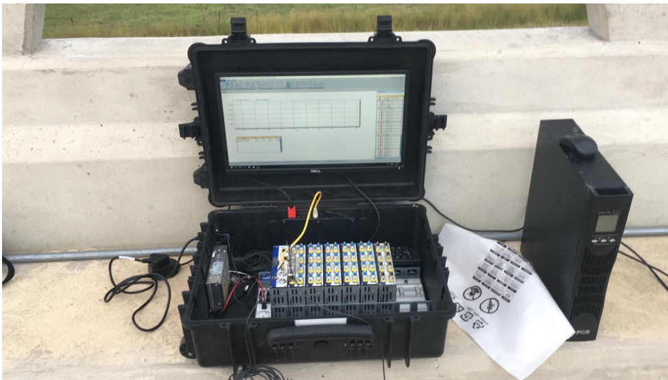
Figure 3.22: HBM QuantumX Data Logger with CATman software
