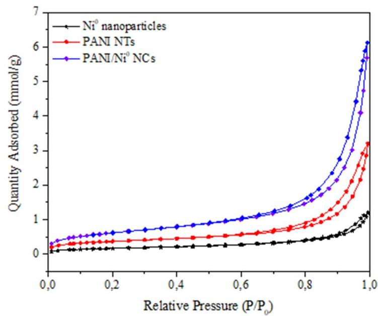
**Fig. S1.** N<sub>2</sub> adsorption-desorption plots of Ni<sup>0</sup> nanoparticles, PANI NTs and PANI/Ni<sup>0</sup> NCs
