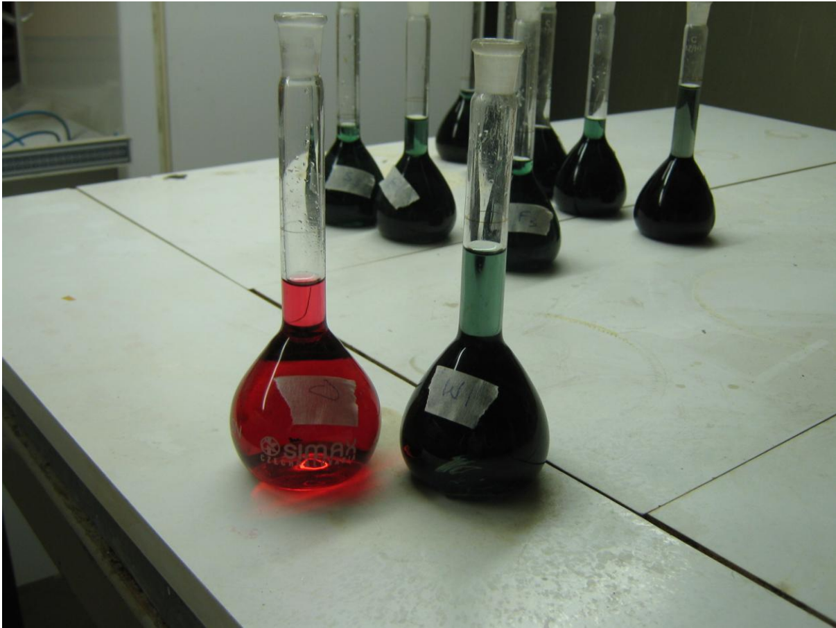
Fig 7.2 Volumetric flasks showing dark green colour change indicative of ammonia volatilization. In contrast is one volumetric flask from an empty jar used to estimate the ammonia content of the introduced air.
