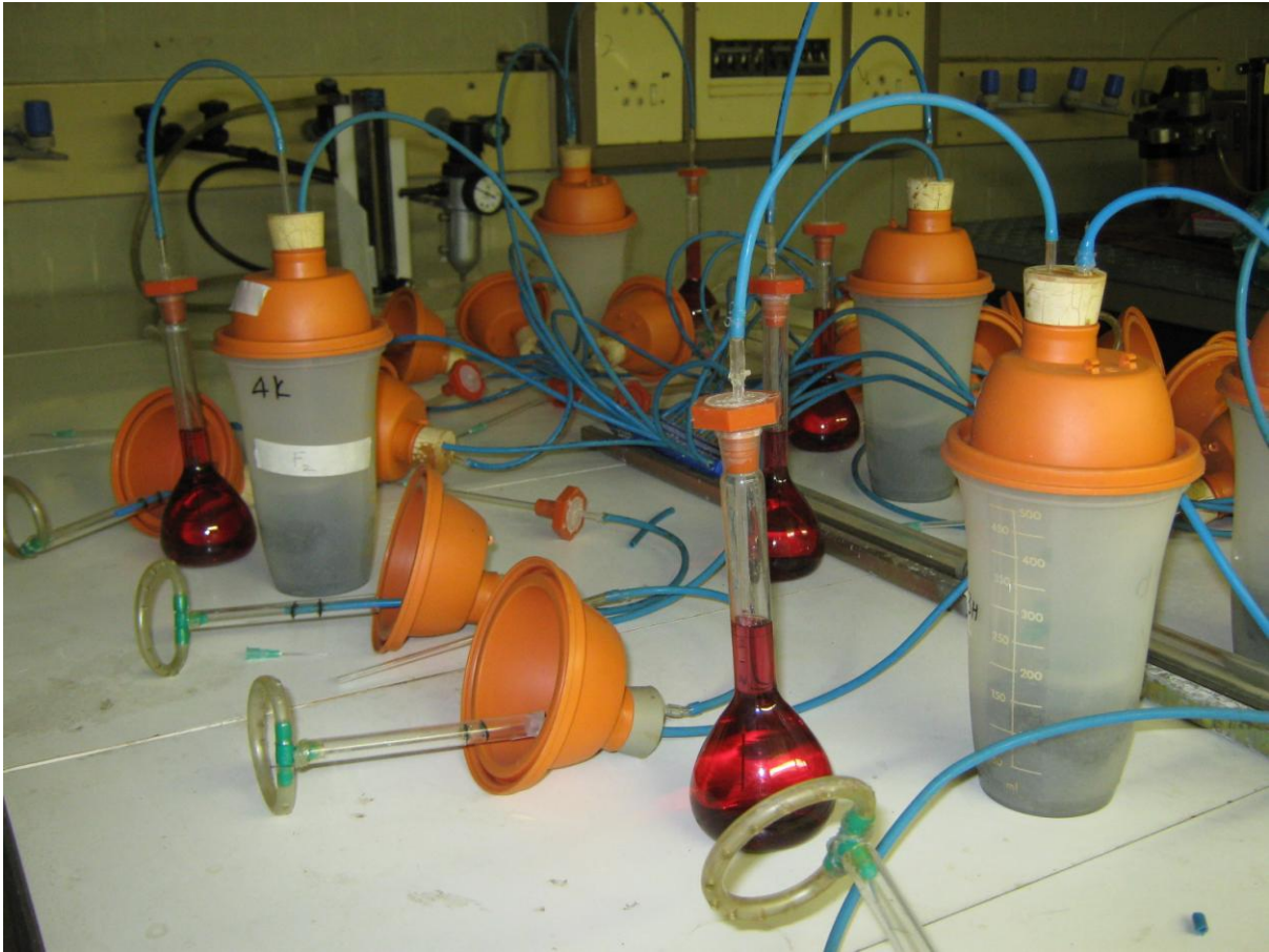
Fig 7.1 Volatilization chamber showing jars, volumetric flasks containing boric acid solution with mixed indicator (bromocresol green and methyl red) and airflow compressor.
