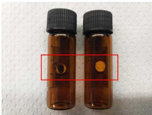
Figure 7: Quartz fibre filters used to collect particulate emissions for the EUR10 fuel during the low phase of the WLTC test cycle with the DOC only (left) and the DOC-DPF (right) in-line.
