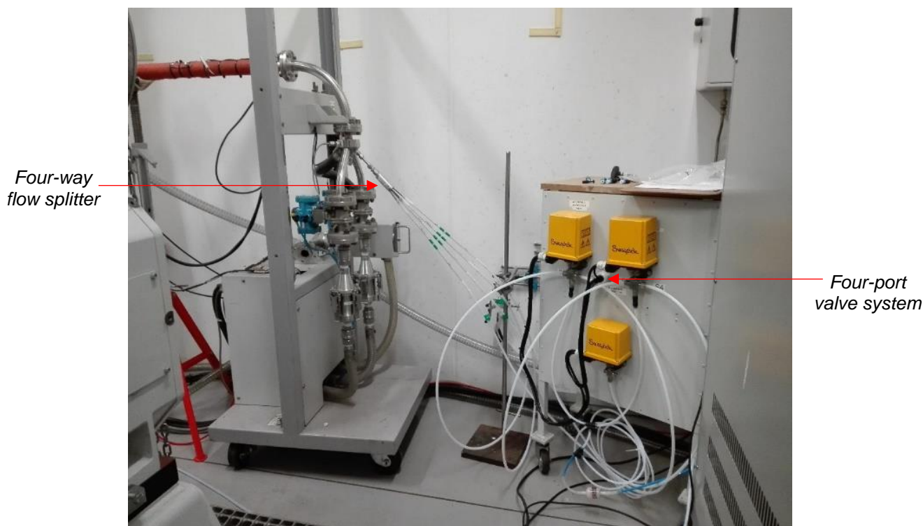
Figure 3.8 Sampler setup during the transient cycle emissions tests.
