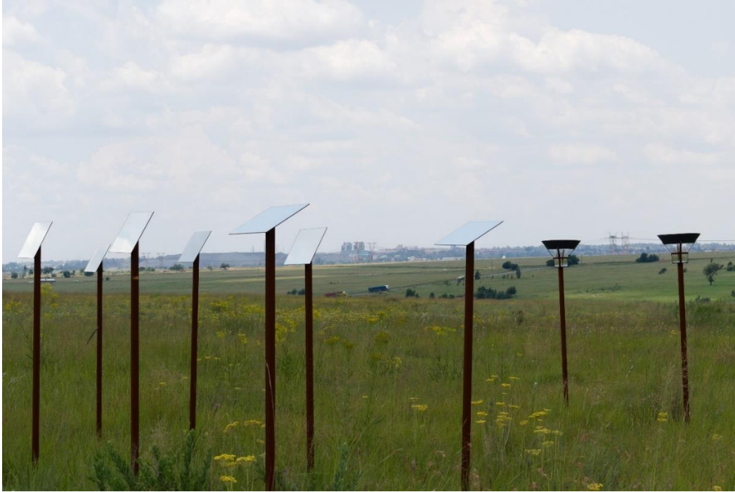
Figure 13. Reflector sampling set four (S4), consisting of eight reflectors, six of which are elevated at 60° and two at 30°. Two collocated dust deposition samplers are seen in the background. The ferrochrome smelter is seen in the far background centre.
