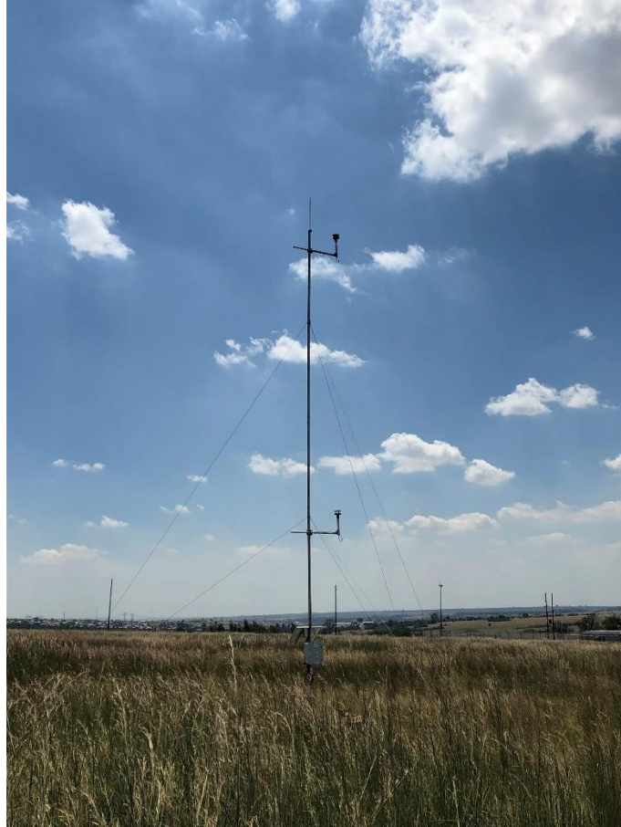
Figure 12. Wind mast with two 2-dimensional ultrasonic anemometers, one at 4 m and one at 10 m height AGL.
