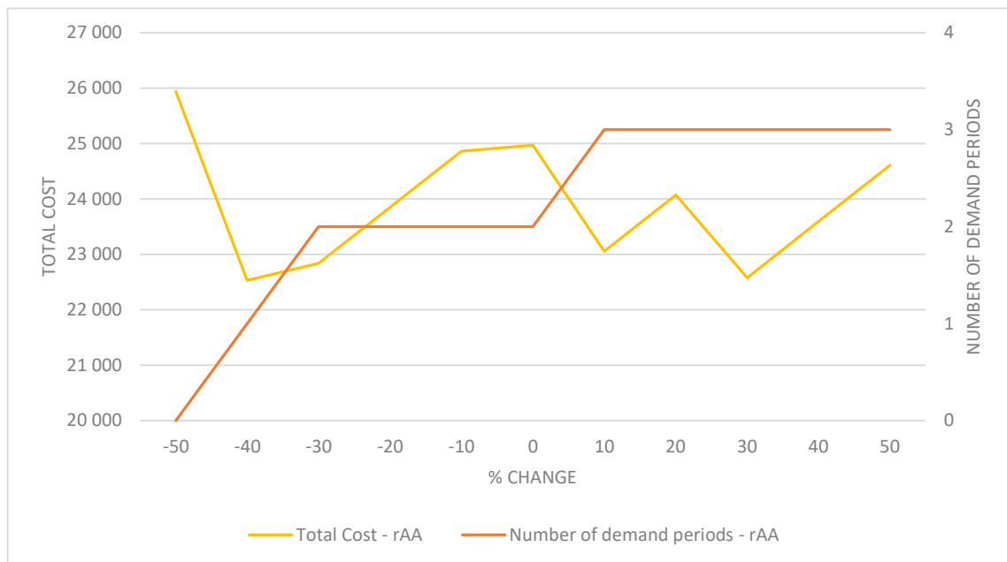
FIGURE 3.4 IMPACT OF CHANGE IN TYPE A RETURN RATE ON TOTAL COST AND NUMBER OF DEMAND PERIODS FULFILLED BY REMANUFACTURING
