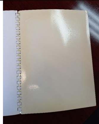
Figure 9: Image showing signs of acid migration on the cover of the volume and close to the combed binding
