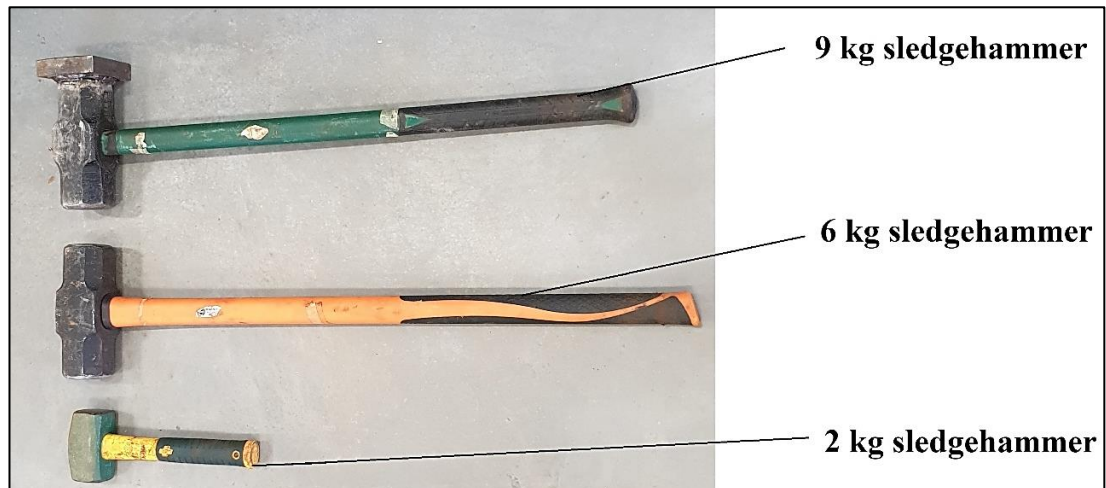
Figure 3.21: Sledgehammers used for conducting the SASW tests.
