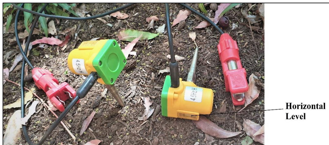
Figure 3.23: Horizontal geophone 4.5 Hz for Love wave tests.
