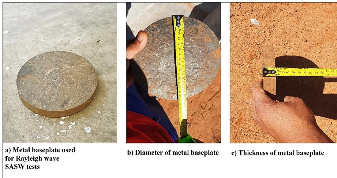
Figure 3.19: Characteristics of metal striking baseplate.
