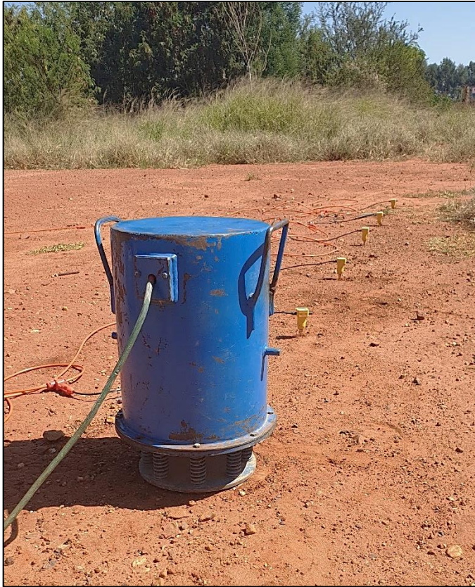
Figure 3.11: High Frequency Shaker (Rayleigh Wave CSW test configuration).
