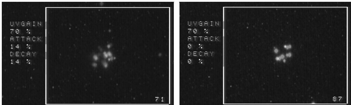
Figure 4.2. Single frame attack and decay on (left) and attack and decay off ( right).
