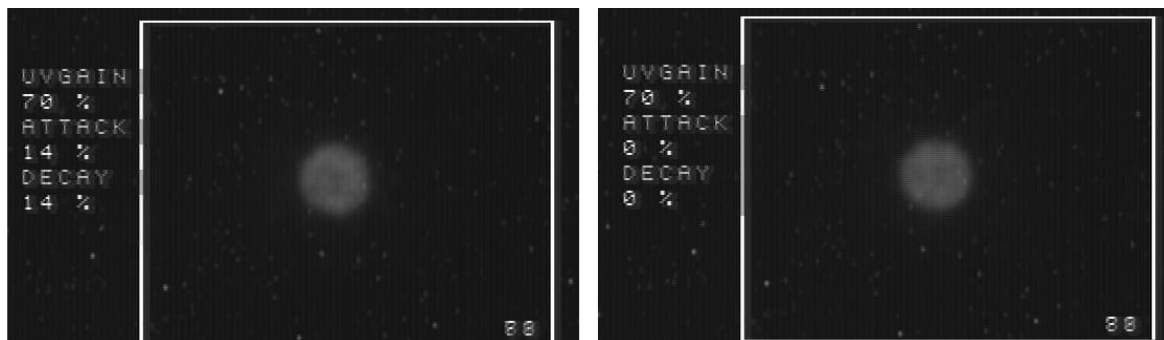
Figure 4.3. Summation of 200 frames with attack and decay on (left) and the summation of 200 frames with attack and decay off (right).
