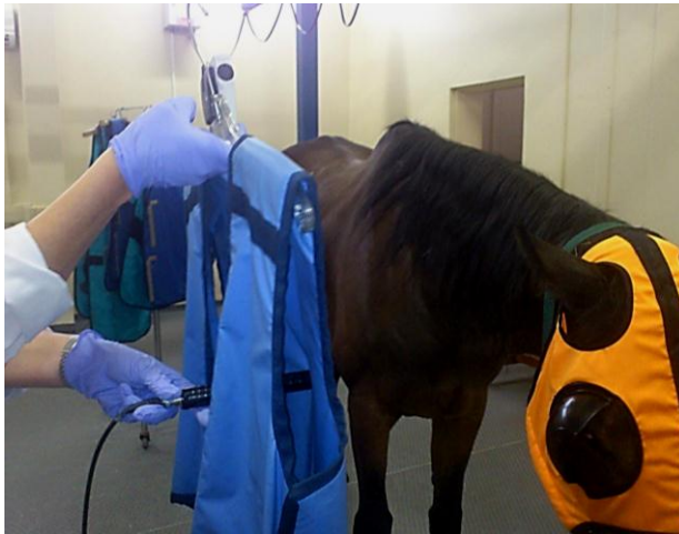
Fig 10. Spectrometer recordings behind lead aprons of varying thicknesses with no additional shielding on the
