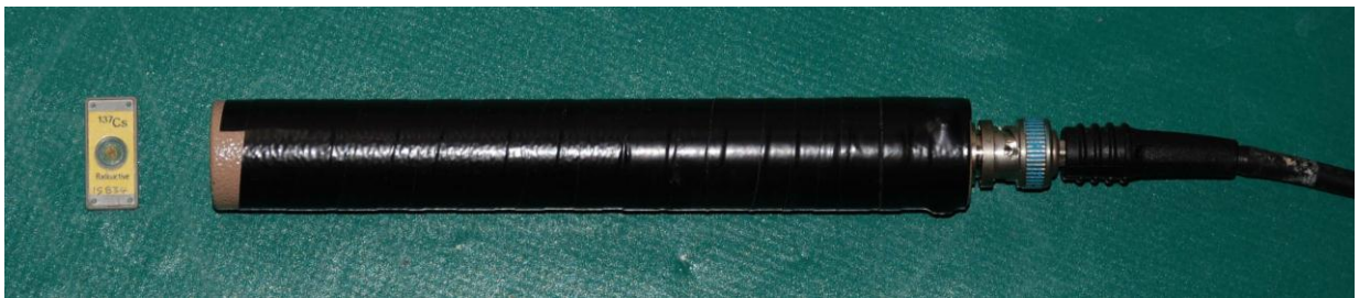
Fig 7. The portable NaI:Tl spectrometer detector.
