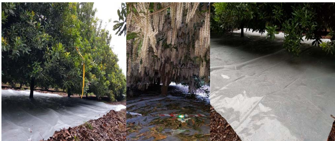
Figure 3.4 Implementation and placement of 200 µm clear plastic rain-covers beyond the 32m 2 allocated to each treatment tree in order to implement water deficits during different phenological stages by eliminating unwanted soil water replenishment
