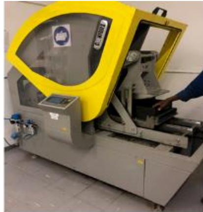
(b) Slab Roller compactor
