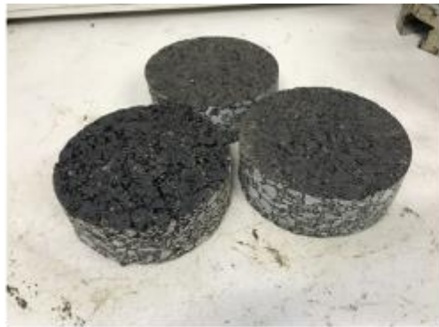
a) RSST-CH test specimens
