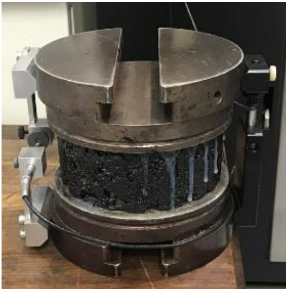
Figure 3.27: The RSST-CH test set-up
