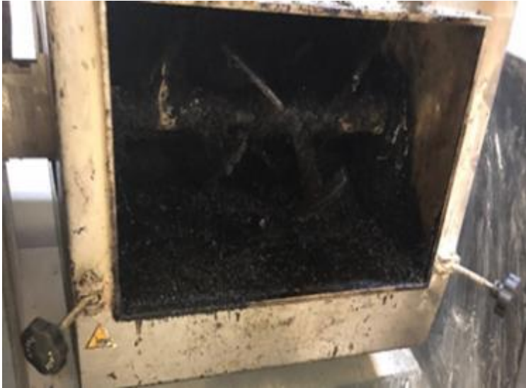
Figure 3.4: Mechanical HMA mixing
