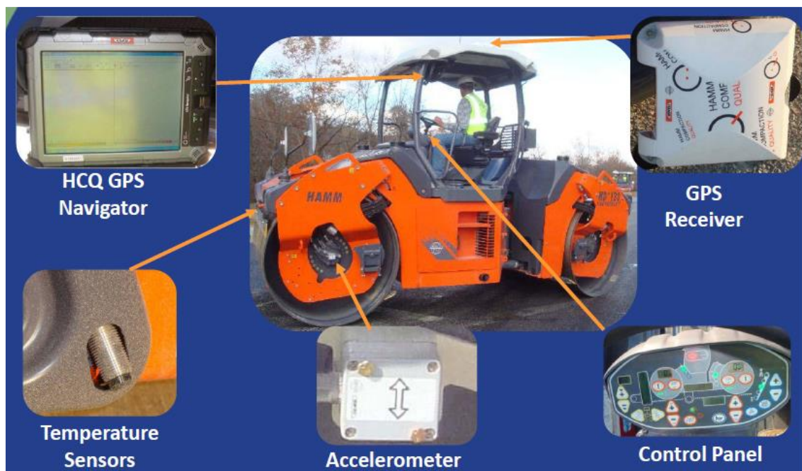
Figure 2.18: Functioning of Intelligent Compaction roller (FHWA, 2014)
