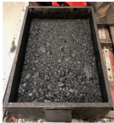
b) Slab roller compacted sample
