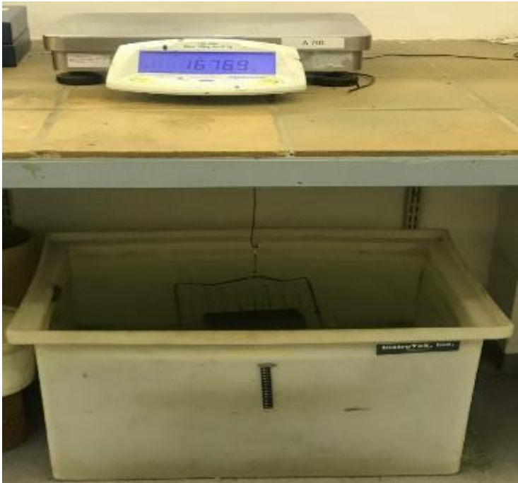
Figure 3.15: SSD test set-up
