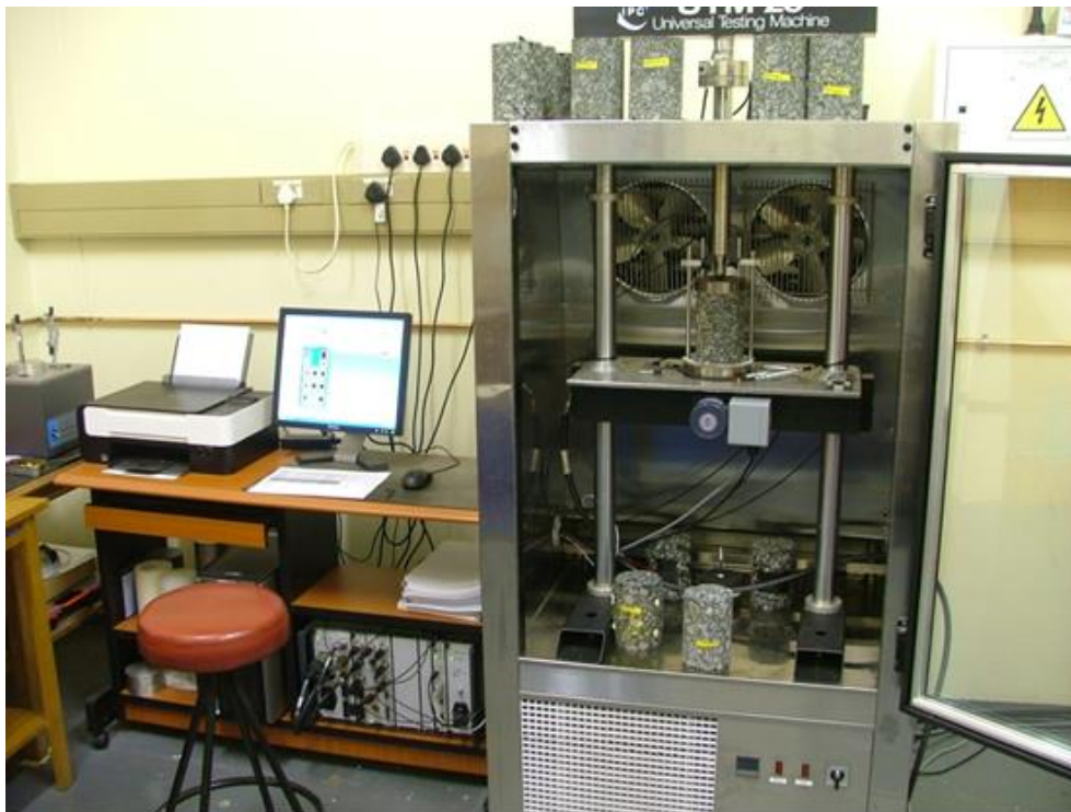
Figure 2.26: RLPD test set-up at the CSIR
