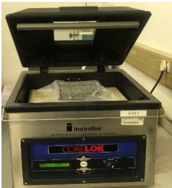
Figure 2.20: Set-up for vacuum-sealing method
