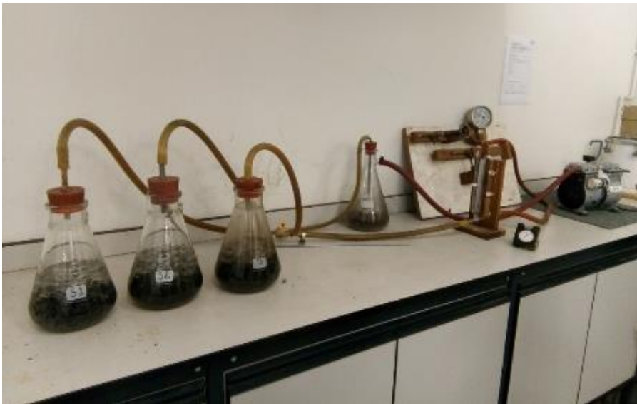
Figure 3.16: MVD test set-up
