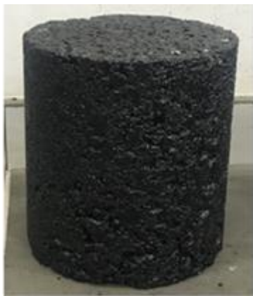
a) Gyratory compacted sample
