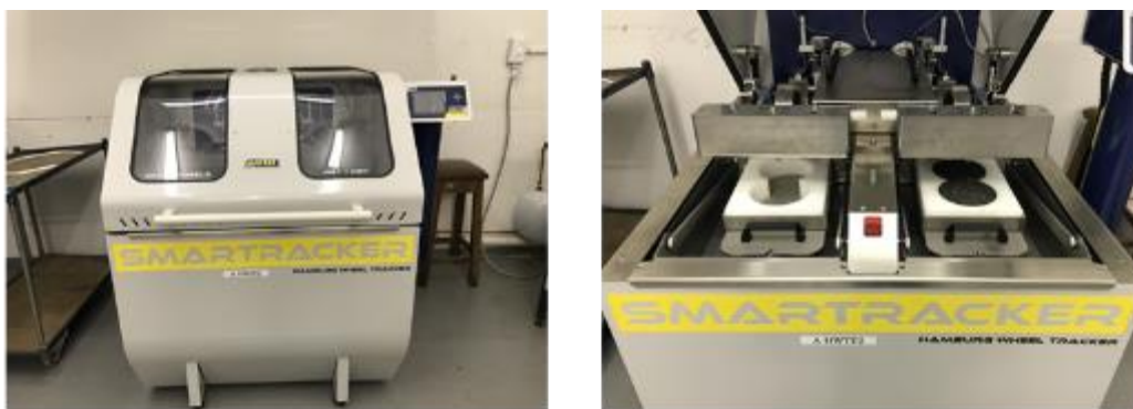
Figure 2.25: Hamburg Wheel-Tracking Device (HWTD)
