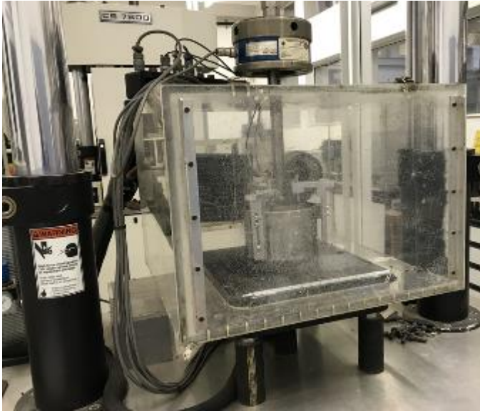
Figure 3.28: UST temperature conditioning chamber
