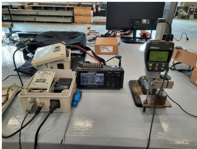
Figure F.1: Calibration of LVDTs using a precision scale
