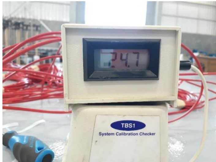
Figure F.3: Calibration system used to calibrate thermocouples
