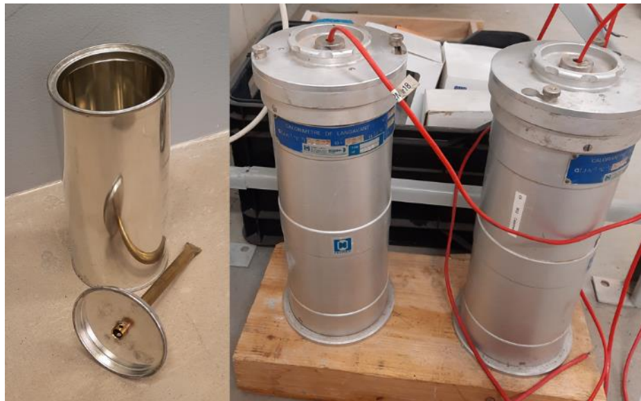
Figure 3.1: Semi-adiabatic calorimetry setup with (Left) the sealable cylinder and (Right) a Dewar flask
