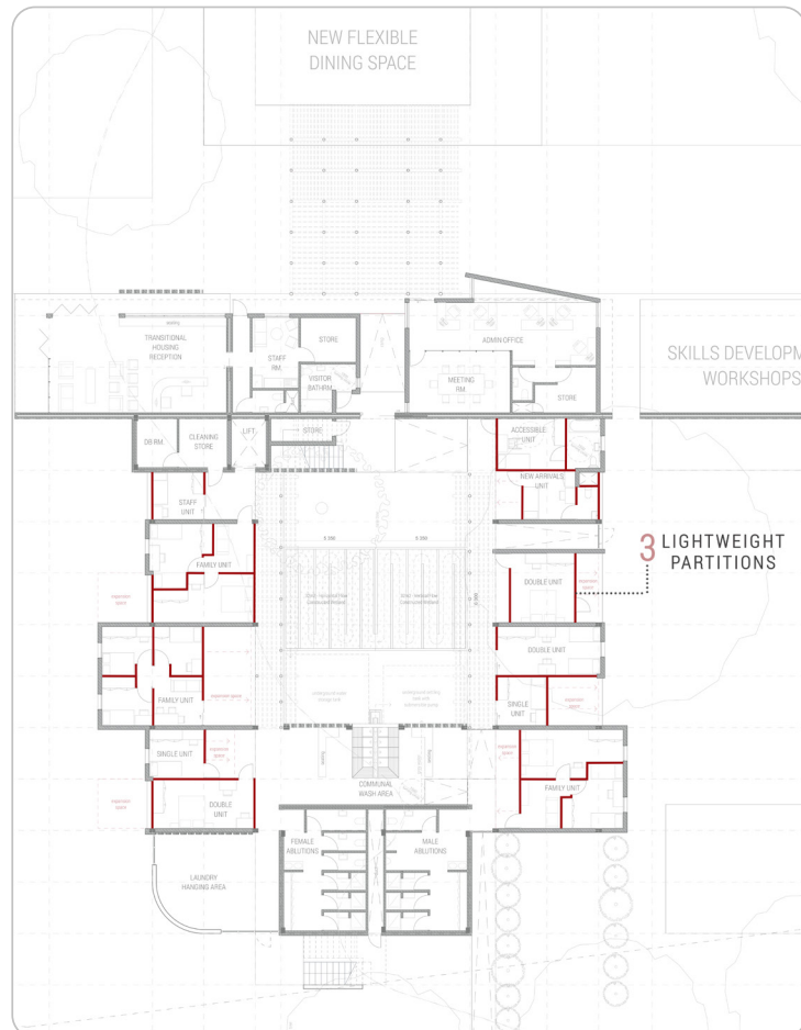
18.14. Cluster A key plan showing lightweight infill panels and partitions of level 3 on the SOP (Author 2021).
