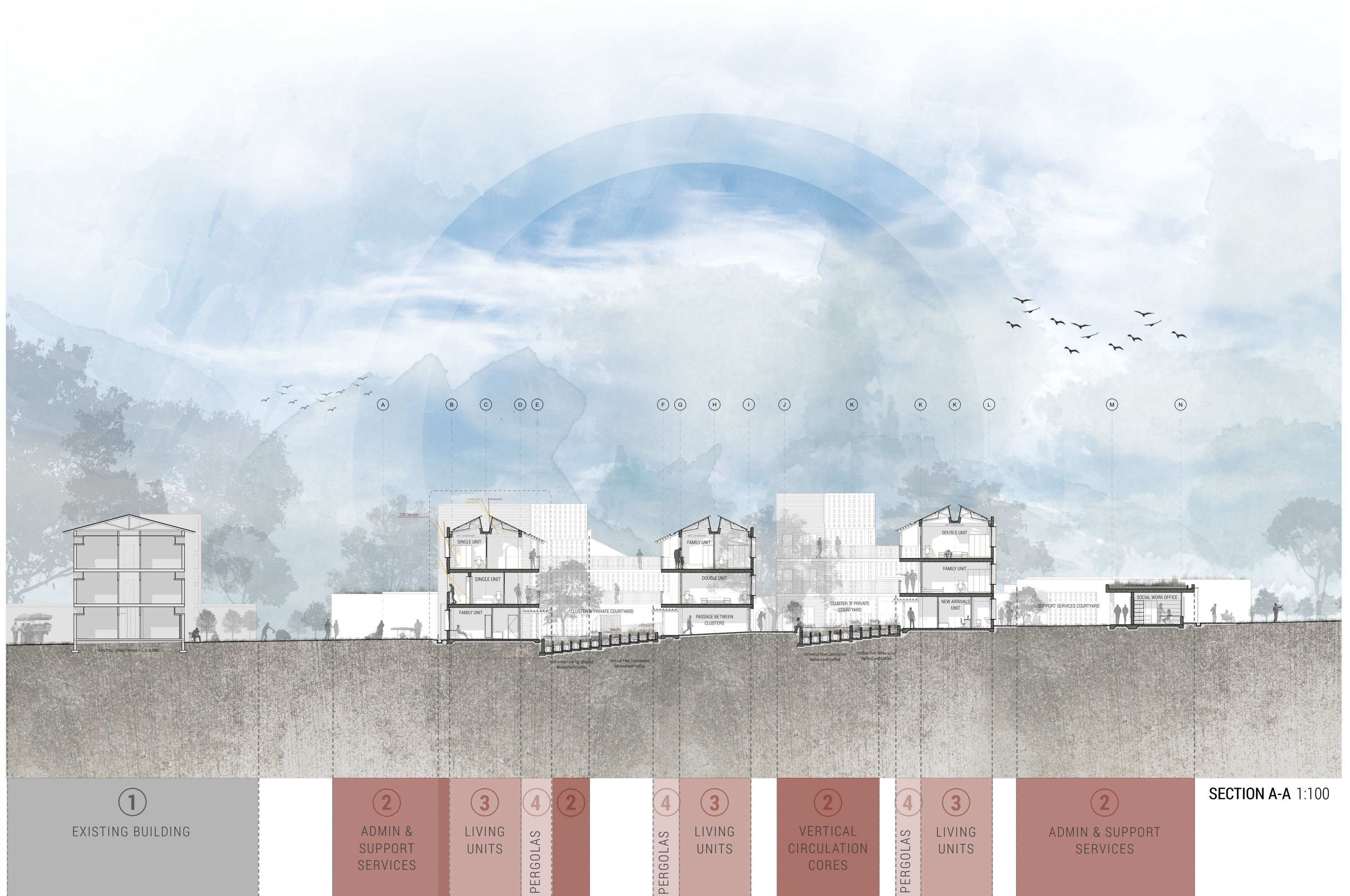
Final Section A-A at scale 1:100 on A0 landscape, indicating various spaces according to their levels of permanence (Author 2021).
