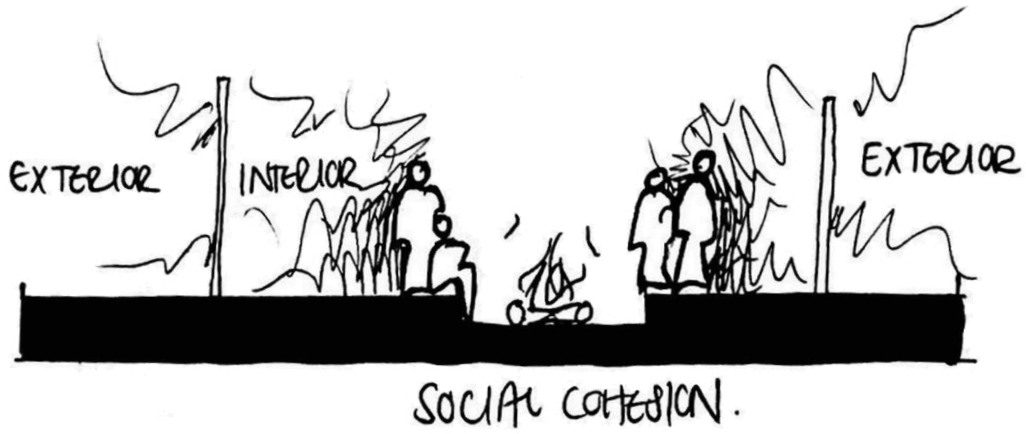
Figure 39: Diagrammatic representation of the typical layout of a communal fire space found throughout the settlement. The spaces are made up of a centralised fire pit with seating and a barrier between the space and its surroundings. This becomes a key informant going into the design phase of the project (Author, 2021).
