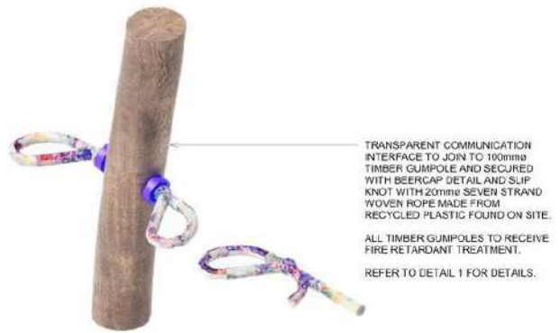
DETAIL 2 JOINT DETAIL
