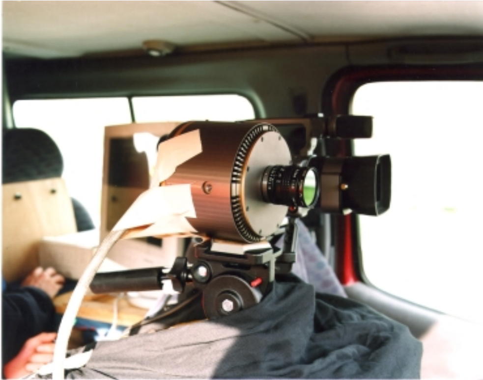
Fig. 5 Measuring the visibility with a special scientific video camera from inside a vehicle.
