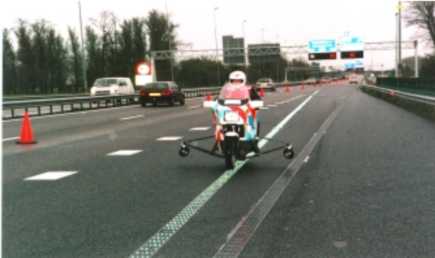
Fig. 4 Measurement of brake delay with motorbike without ABS
