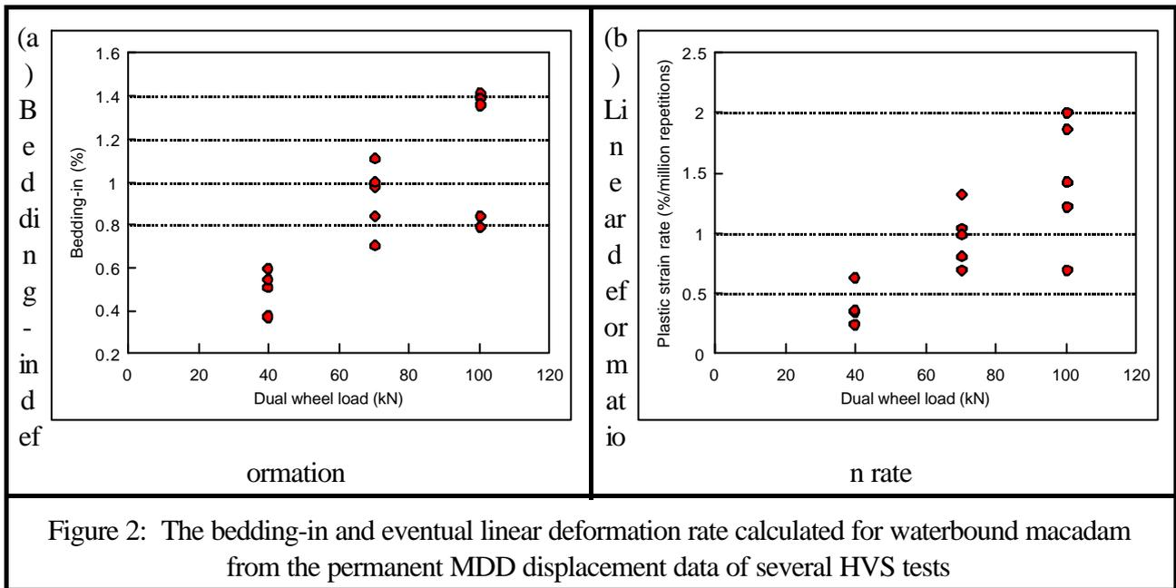
Figure 2: The bedding-in and eventual linear deformation rate calculated for waterbound macadam from the permanent MDD displacement data of several HVS tests
