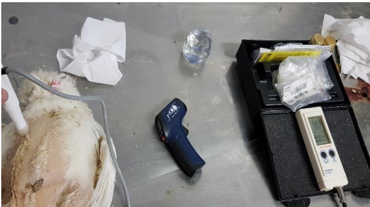
Figure 3.3.1.1: Carcass pH and temperature recordings during decomposition trial. Each carcass collected during the decomposition trial was recorded for carcass pH and temperature after the designated time intervals (FRESH=0h, CAR1=6h, CAR2=12h, CAR3=18h, CAR4=24h, SEVROT=36h).
