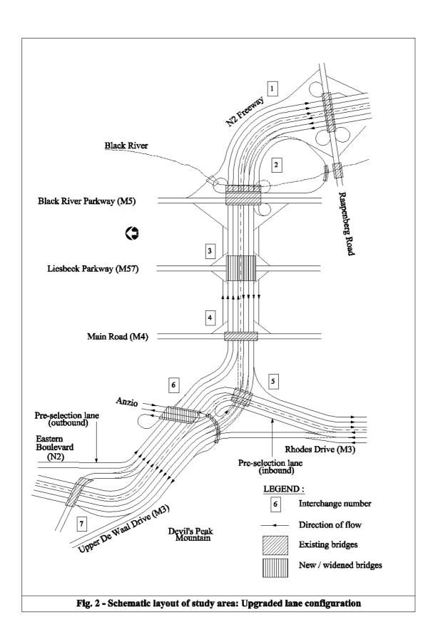
It was therefore decided to use the opportunity presented by the under-utilised on-ramp at Raapenberg Road and construct a new ramp from the M5 to the N2. The area between the M5, N2 and the new ramp was as the same time reclaimed as a wetland. The existing loop ramp was closed and demolished. The new ramp presented design challenges as there was both vertical and horizontal deviation.
