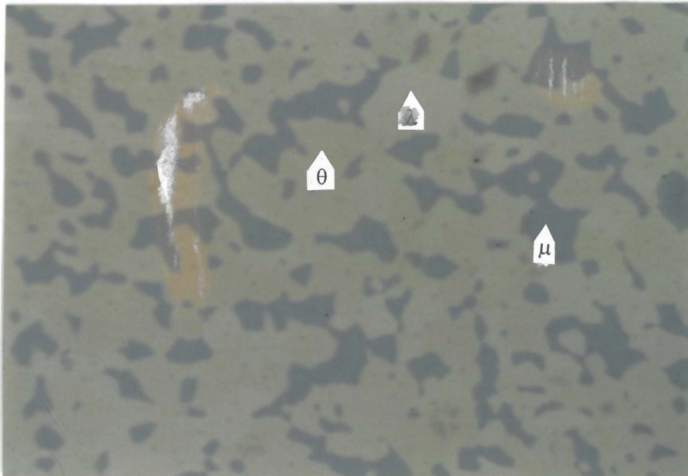
Photomicrograph 16. Intergrowth of \text{Cu}_{2-x}\text{S} ( \mu , grey) + \text{Ni}_{1-x}\text{S} ( \lambda , light yellow) + \text{Ni}_{3\pm x}\text{S}_2 ( \theta , darker and lighter yellow). It is not possible to distinguish between \text{Ni}_{1-x}\text{S} and \text{Ni}_{3\pm x}\text{S}_2 on the photograph, due to their similar colours. Charge 267, at 700°C, (long side of the photomicrograph is 250 \mu\text{m} ).
