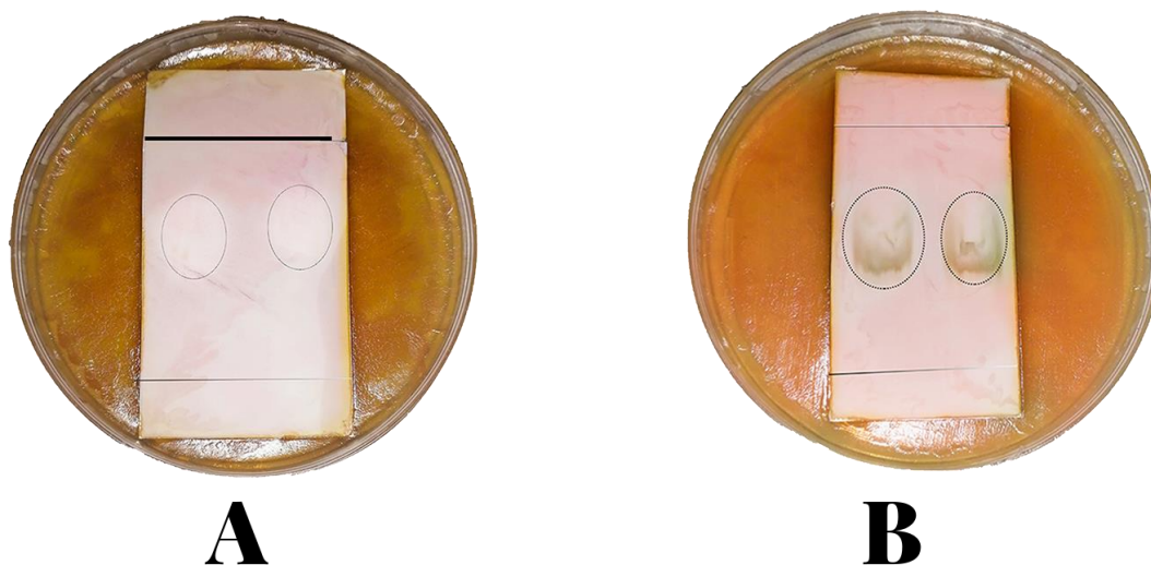
Figure 4.7. TLC bioautography of (A) S. aromaticum hexane extract and (B) C. sativum hexane extract. (A) No specific band could be seen but only a zone of inhibition was observed from 32mm (circled). The Rf value calculated from this result was 0,64. (B) Two major bands can be seen from 29mm (circled). The Rf value calculated is 0.58
