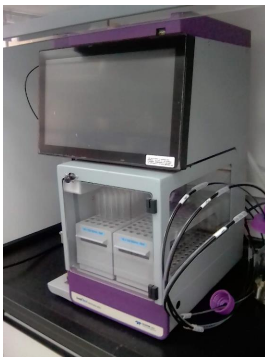
Figure 5.8: Automated flash chromatography system with UV-VIS detector.
