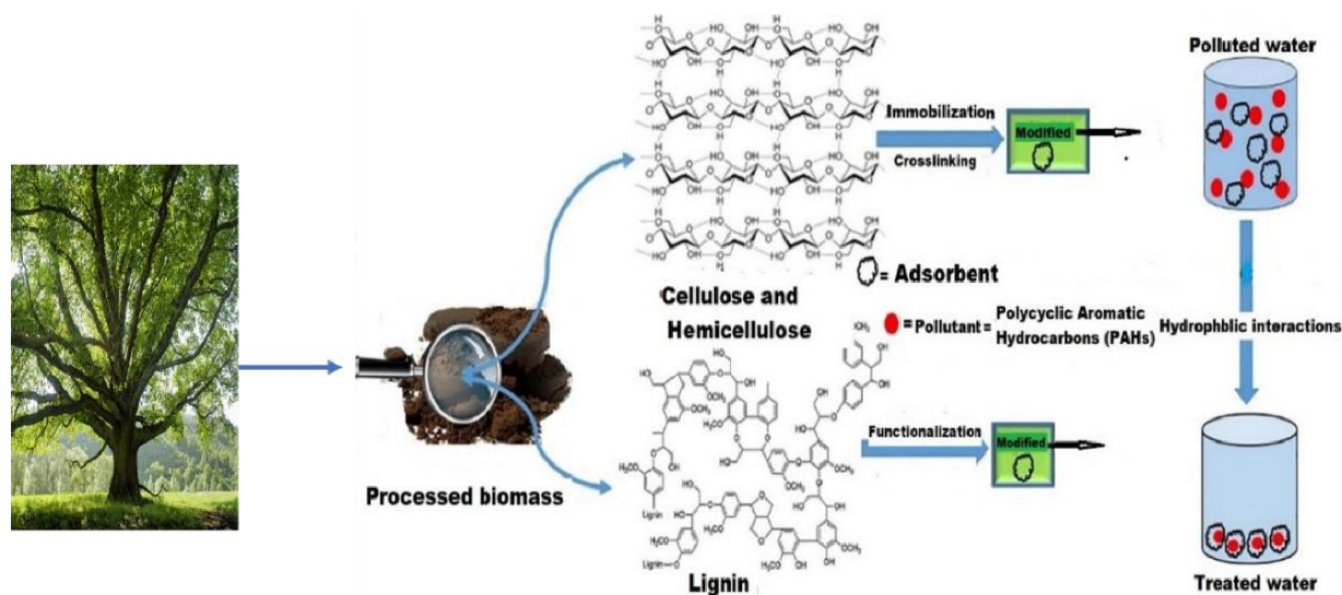
Figure 3. Treatment of PAH-contaminated water using plant derivatives (biomass).
