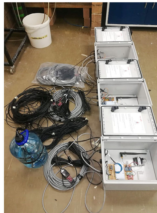
Figure 3 DAQs and sensors preconfigured in the laboratory
