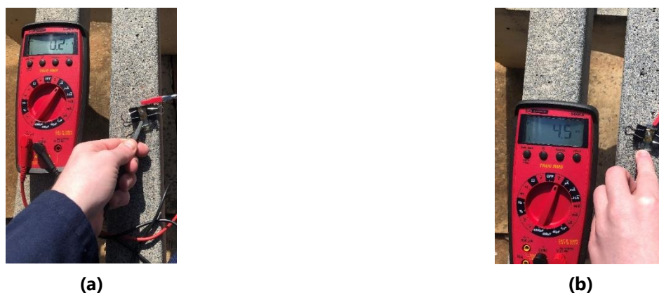
Figure 6.11 (a) The maximum current measurement and (b) the maximum voltage measurement of the PSC device FTO/ D-NaBr 3 /MAPbI 3 /CuSCN/Carbon/FTO.
