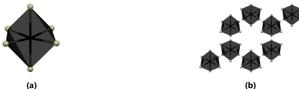
Figure 1.13 (a) Isolated \text{PbBr}_6 octahedron and (b) the isolated \text{PbBr}_6 octahedra as viewed down the c -axis of the structure \text{DPbBr}_6 . Cations are omitted for clarity.
