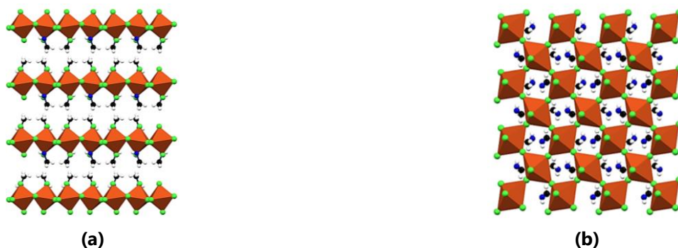
Figure 1.7 The crystal structure of \text{MA}_2\text{CuCl}_4 (2D perovskite, n = 1 ) as viewed down (a) the a - and (b) the c -axis, respectively.
