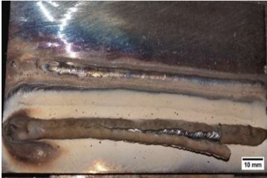
Figure 4.1: Photograph of the LAB 104 bead on plate weldability test showing a combination of sticky (beginning) and splitting slag (centre). The discolouration was visible on the weld bead.
