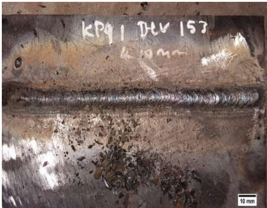
Figure 4.2: Photograph of the LAB the153 bead on plate weldability test showing sticky and difficult to remove slag.
