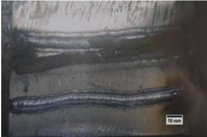
Figure 4.3: Photograph of the LAB 24 bead on plate weldability test showing tendency to self-lifting and splitting slag.
