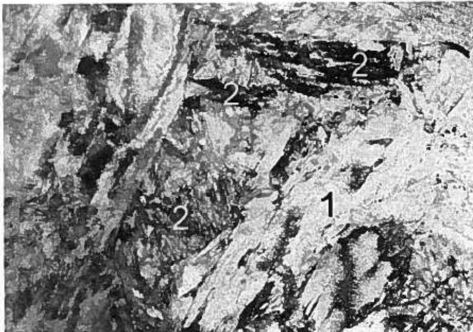
Figure 5.1: Microstructure of P91 (a) simulated reheated coarse grain heat affected (SRCGHAZ) zone X5000 [52].
