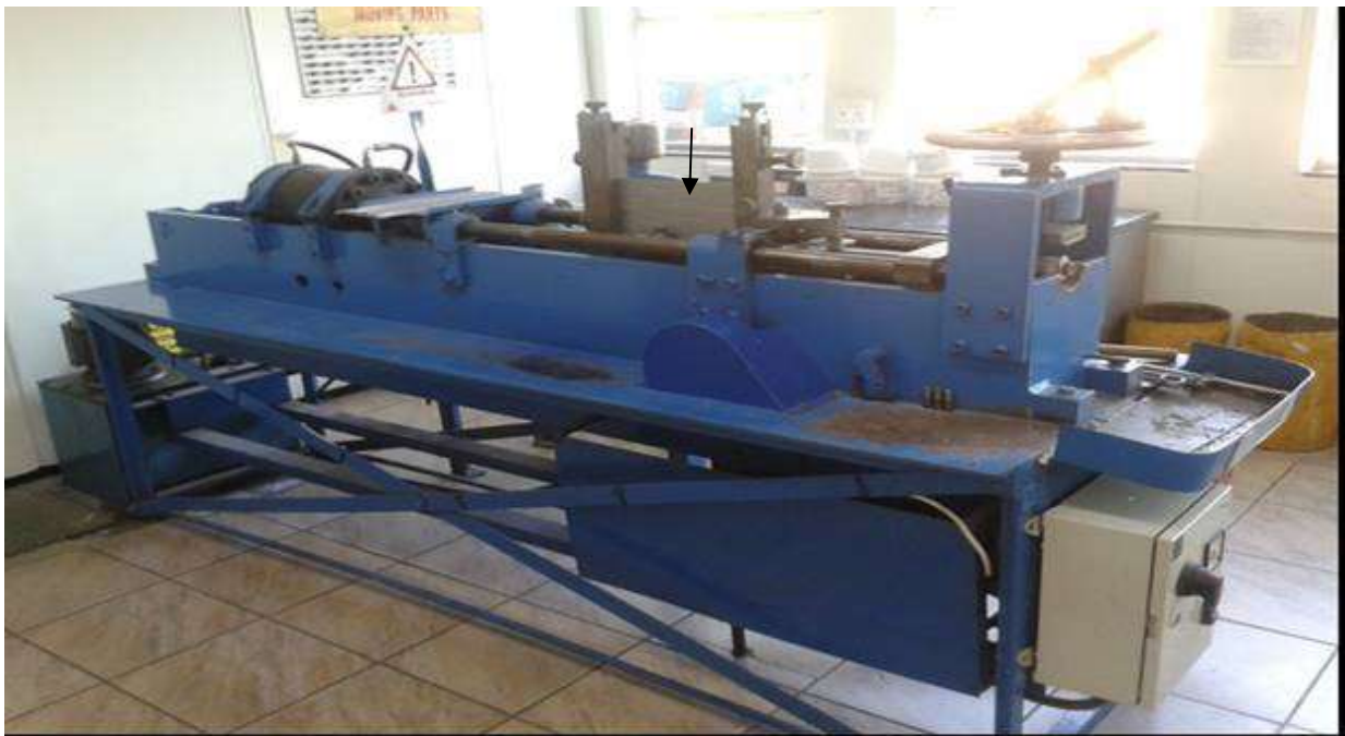
Figure 3.2: Laboratory extruder. Arrow indicates a wire feeder unit.
