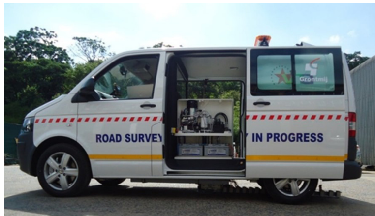
Figure 4: FWD with Internal Deflection Measurement Mechanism
