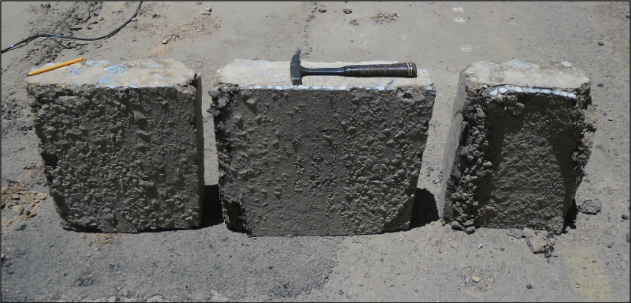
Figure 2: Test-pit blocks cored directly from the NME base layer at Provincial Road D1884
