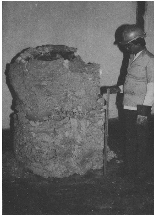
Figure 5: Two-ton block of titanium sponge (Source: Subramanyam, 1993: 446)
