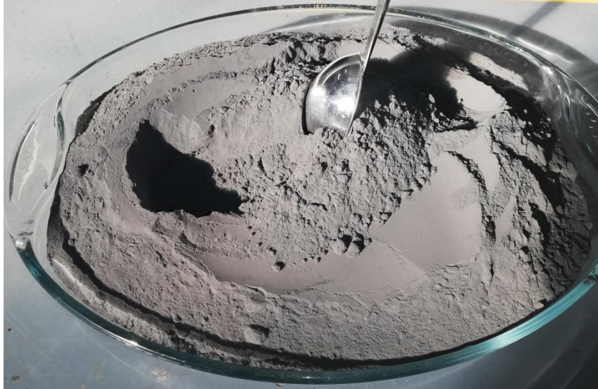
Figure 70: Titanium metal powder produced during the experiment
