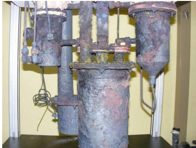
Figure 58: Photograph of a reactor prototype with excessive corrosion damage
