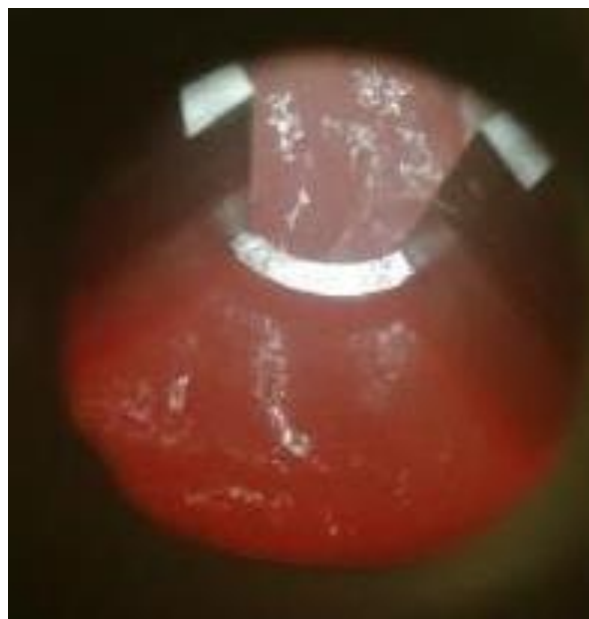
Figure 54: Photograph showing molten salt flow inside an operational reactor
