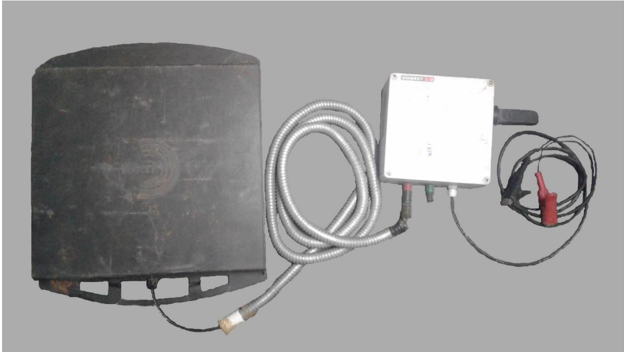
Supplementary Figure 3: RFID reader array with a custom made decoder LID650/608 (DorsetID, Aalten, Netherlands) attached to the panel antenna ANT612. The black panel scans for passive integrated transponder tags at regular intervals which are stored on a USB drive attached to the white recording box. Red and black cables are attached to a power source.
