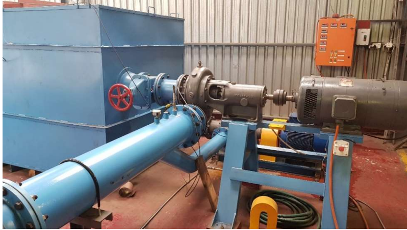
Figure 4-19: Two centrifugal parallel connected centrifugal pumps
