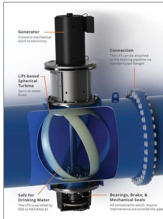
Figure 2-11: Blade-type turbine produced by Lucid Energy (Lucid Energy, n.d.)
