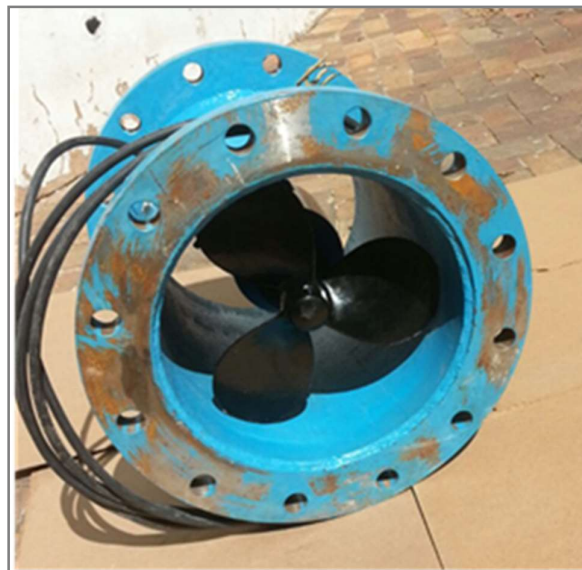
Figure 3-19: AmpAir unit in a spool piece
