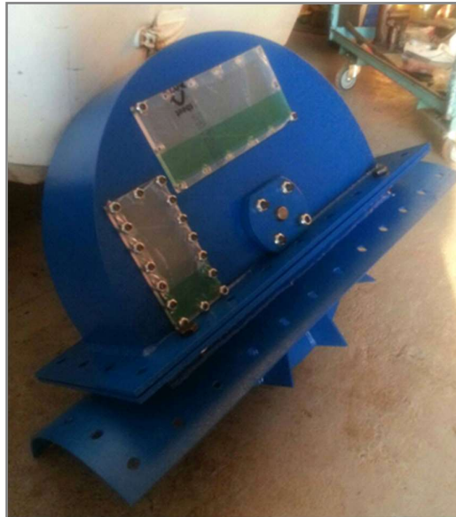
Figure 4-10: Prototype 3 and 4 – runner housing with runner assembling
