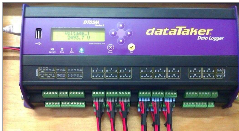
Figure 3-16 : Logging device used during turbine testing
