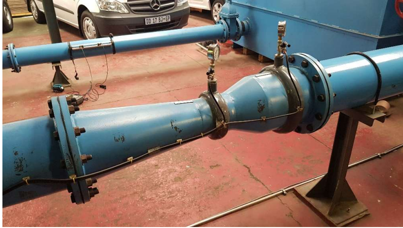
Figure 4-21: A venturi installed as part of the test setup
