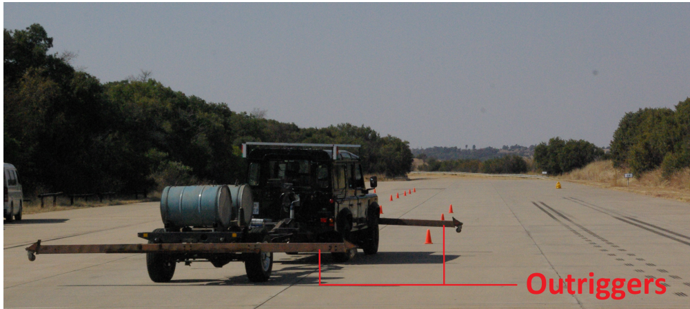
Figure 3.3. Articulated vehicle setup showing outriggers
