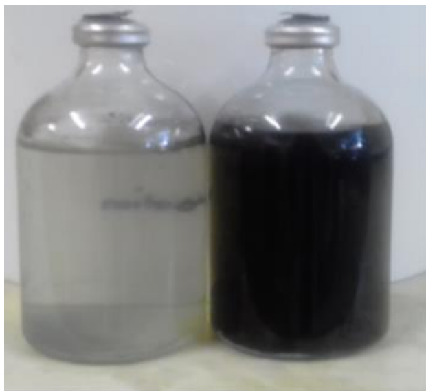
Figure 3. 2: Blackening of the medium due to SRB growth
