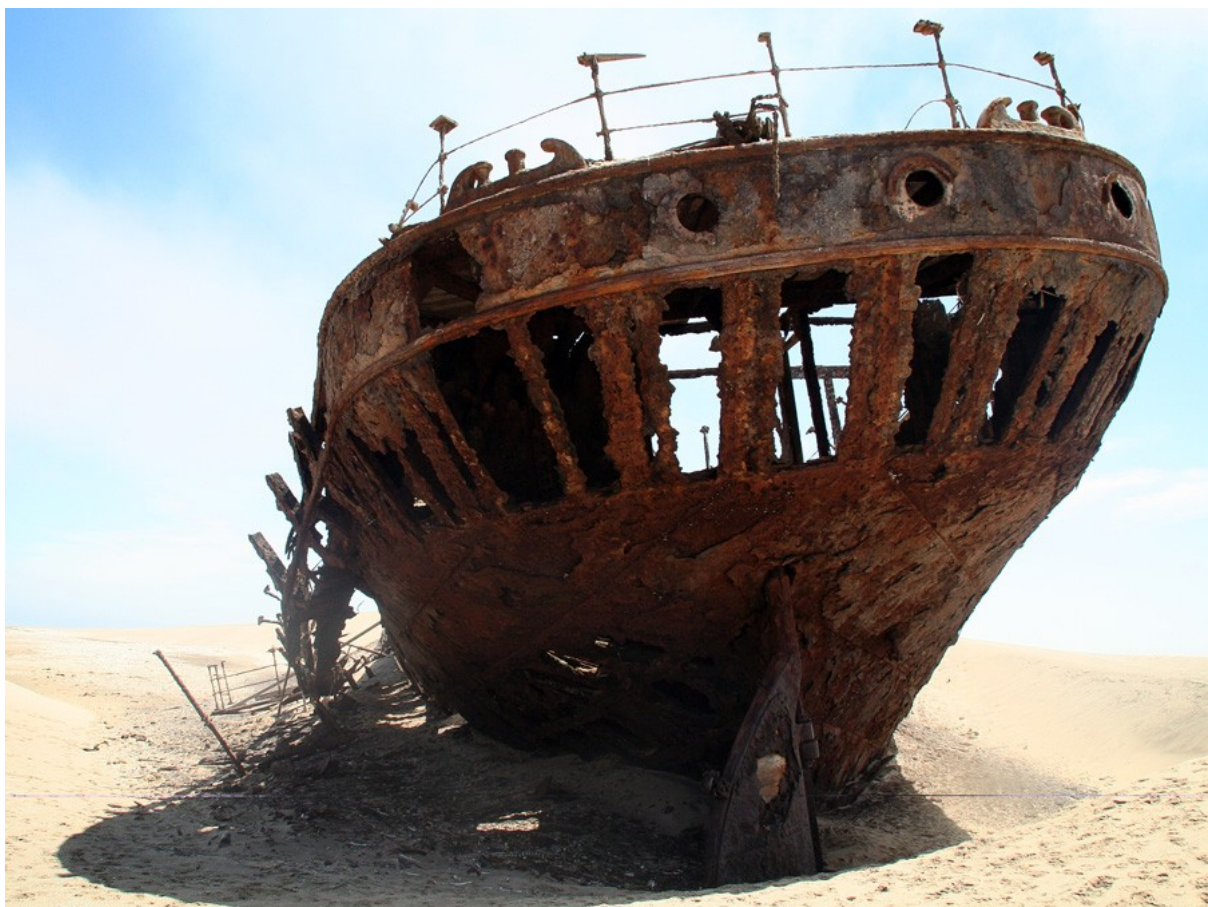
Figure 4.1. Eduard Bohlen has lost its aesthetic value over time due to corrosion (Source: Harris et al. 2012).
